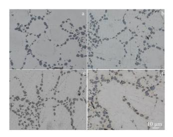
Fig.5 Microstructures of A356 alloy after aging at 180 °C for different time: (a) 2 h, (b) 4 h, (c) 6 h, and (d) 8 h
