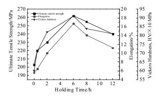
Fig.3 Variation of tensile strength, elongation and Vickers hardness at 540 °C for different solution time
