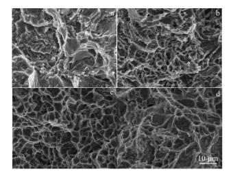
Fig.4 SEM fracture morphologies of solution treated alloys at 540 °C for different time: (a) untreated, (b) 2 h, (c) 6 h, and (d) 12 h
