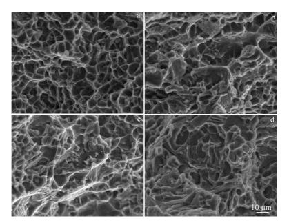
Fig.9 SEM fracture morphologies of alloy after different heat treatments: (a) solution for 6 h; (b) solution for 6 h and aging for 2 h; (c) solution for 6 h and aging for 4 h; (d) solution for 6 h and aging for 8 h
