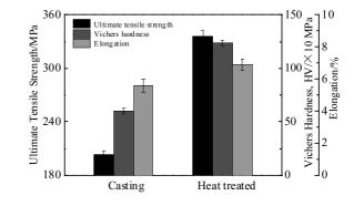
Fig.8 Tensile strength, elongation and hardness of the alloy before and after heat treatment
