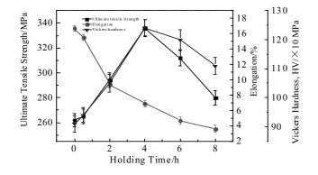
Fig.7 Variation of tensile strength, elongation and Vickers hardness of alloy aging treated at 180 °C for different time
