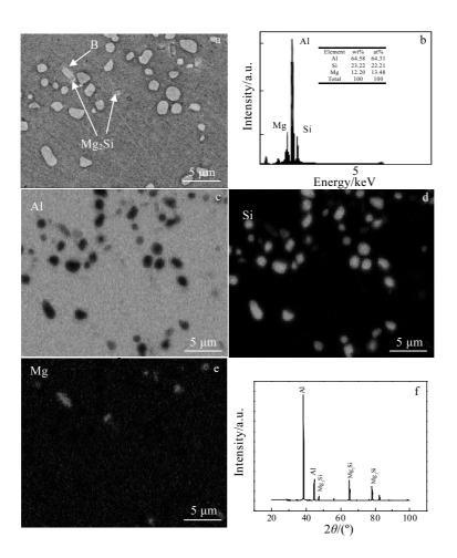
Fig.6 SEM image (a); EDS result of position B in Fig.6a (b); distributions of element Al (c), Si (d), Mg (e); XRD pattern (f) of the alloy aged at 180 °C for 4 h
