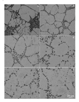
Fig.1 Microstructures of the alloy at 540 °C for different solution time: (a) 0 h, (b) 0.5 h, (c) 2 h, (d) 6 h, (e) 8 h, and (f) 12 h
