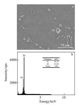
Fig.2 SEM image (a) and EDS result of position A in Fig.2a (b) of the alloy after solution treatment at 540 °C for 6 h
