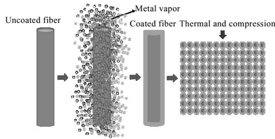
Fig.4 Sketch of MMCs preparation by coating hot pressing technique
