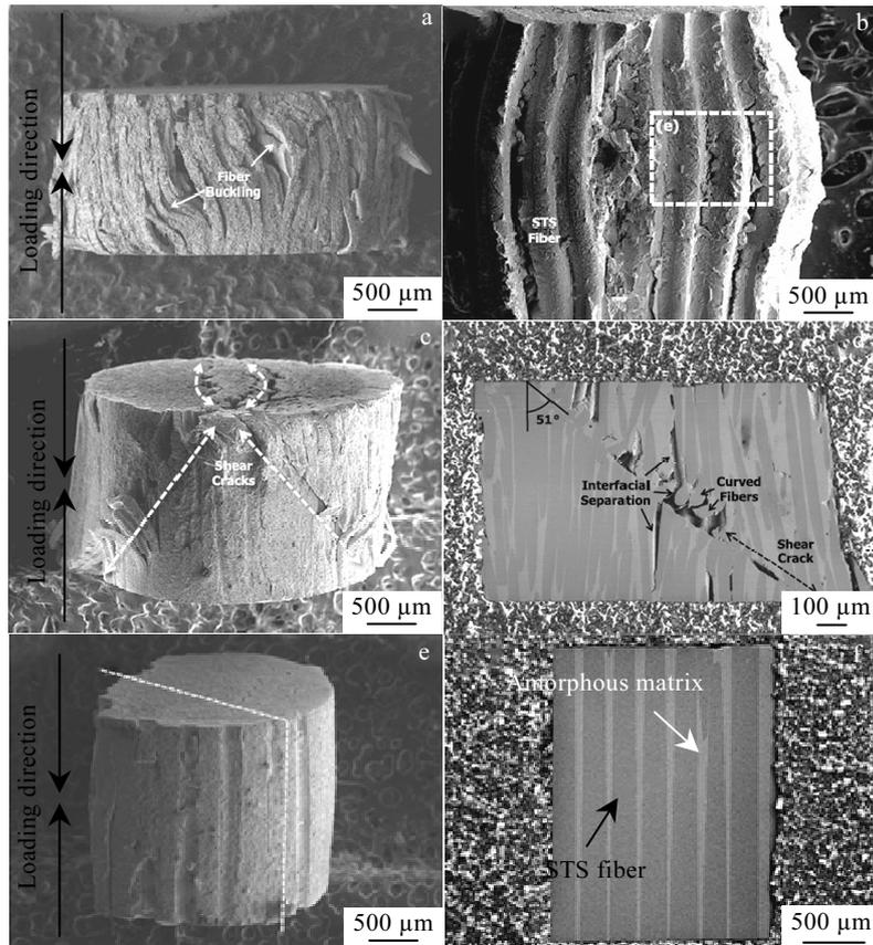
Fig.10 SEM images of deformed compressive specimens: (a) the quasi-statically deformed 110  $\mu\text{m}$ -fiber-reinforced composites, (b) the quasi-statically deformed 250  $\mu\text{m}$ -fiber-reinforced composites, (c, e) the dynamically deformed 110  $\mu\text{m}$  and 250  $\mu\text{m}$ -fiber-reinforced composites, (d, f) cross-section area of the dynamically deformed 110  $\mu\text{m}$  and 250  $\mu\text{m}$ -fiber-reinforced composites<sup>[68]</sup>
