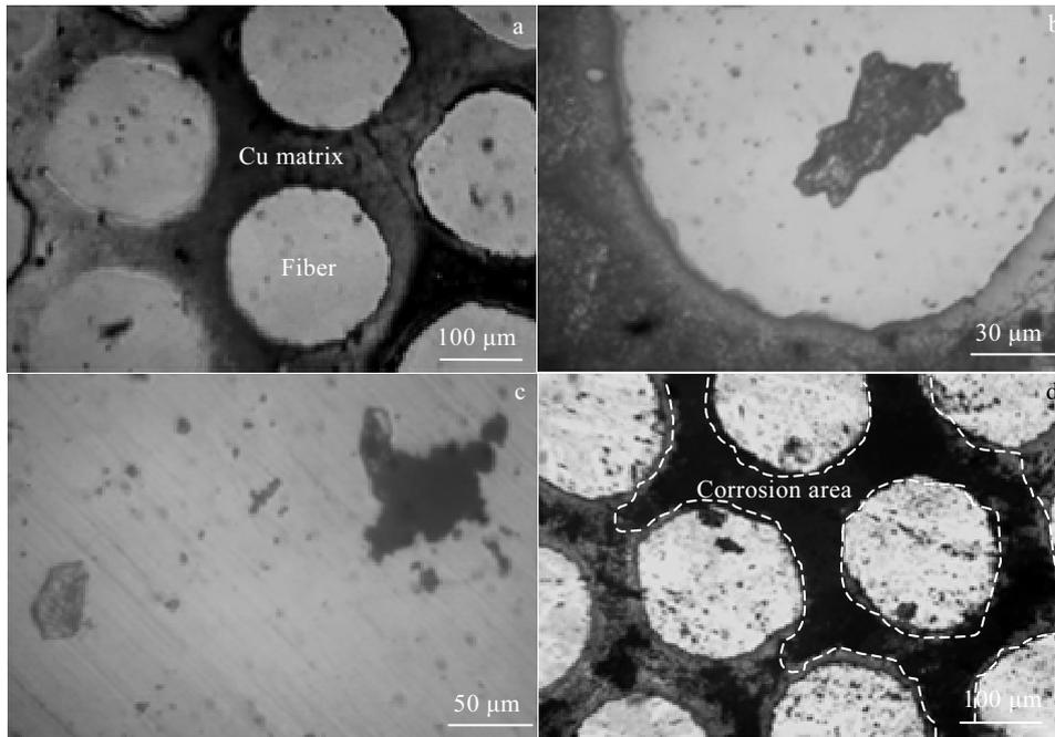
Fig.8 Optical micrographs of corrosion surfaces following free immersion in 30 g/L NaCl solution: (a) stainless steel fiber/Cu MMC specimen for 2 h, (b) stainless steel fiber/Cu MMC specimen for 3 h, (c) monolithic stainless steel specimen for 2 h, and (d) high corroded area in stainless steel fiber/Cu MMC specimen after immersion for 6 h<sup>[59]</sup>
