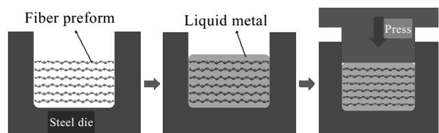
Fig.3 Sketch of composites preparation by squeeze casting technique
