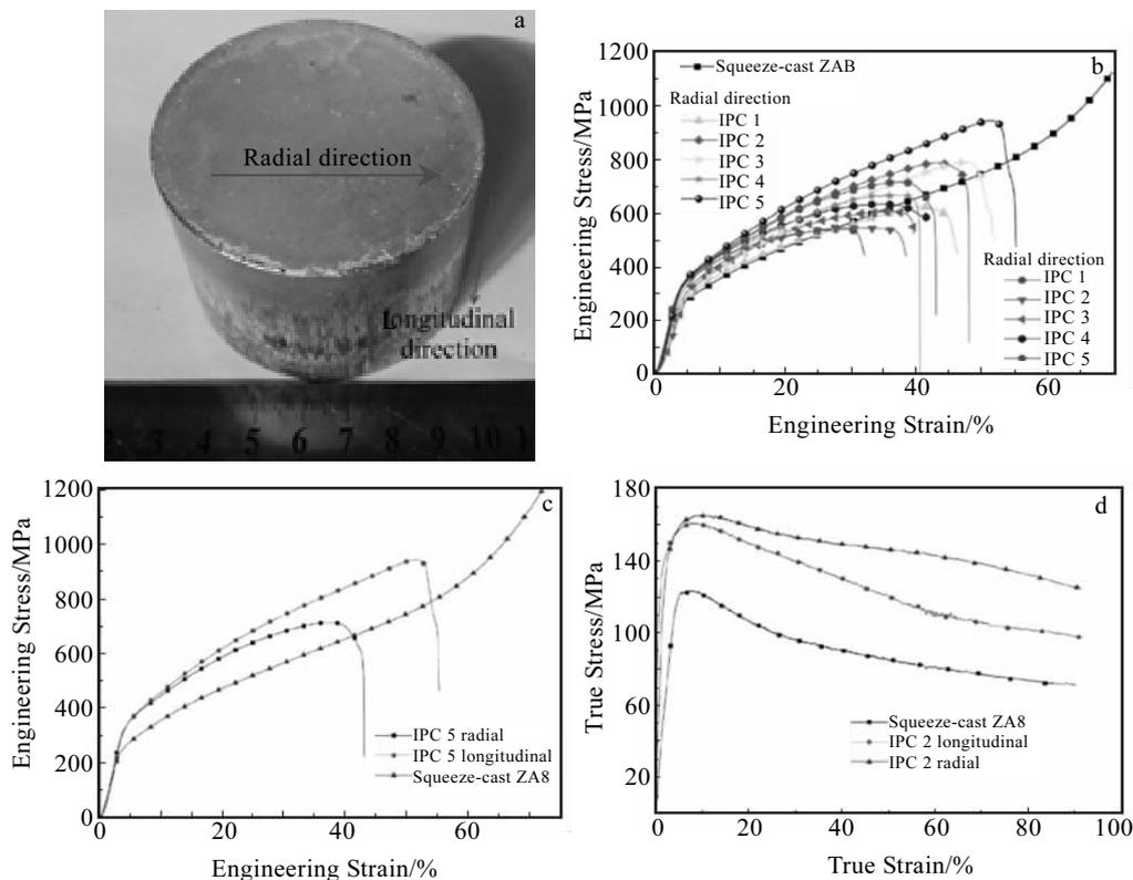
Fig.9 IPCs block sample (a), contrast compressive stress-strain curves of the IPCs in different directions at ambient temperature (b), compressive stress-strain curves of the squeeze-cast ZA8 and the IPCs in radial and longitudinal sections (c), and stress-strain curves during hot compression deformation of the squeeze-cast ZA8 and the IPCs in radial and longitudinal sections (d)<sup>[35]</sup>
