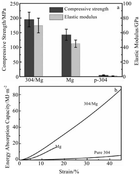
Fig.7 Performance comparison of 304/Mg and pure Mg: (a) compression strength and elastic moduli and (b) energy absorption capacity<sup>[34]</sup>
