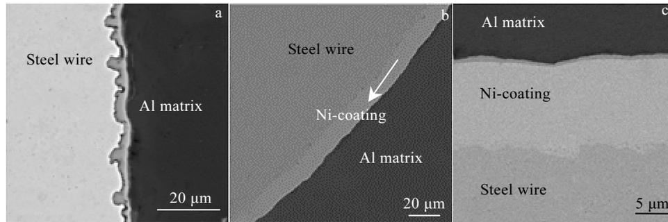
Fig.6 SEM images of Al matrix/steel wire interface in composite: (a) uncoated wire and (b, c) nickel-coated wire<sup>[43]</sup>
