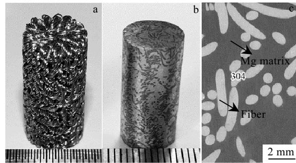
Fig.2 Macrographs of pure 304 stainless steel fiber (a), Mg/304 stainless steel fiber composites (b) and cross section image of composites (c)<sup>[34]</sup>
