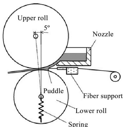
Fig.5 Schematic illustration of the DMDTRC<sup>[39]</sup>
