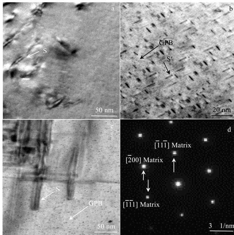
Fig.4 TEM bright field images (a~c) and SAED pattern (d) of C alloy after aging at 175 °C for different time: (a) 6 h, (b, d) 96 h, and (c) 240 h
