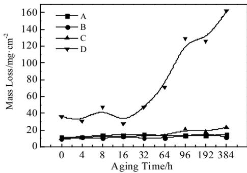
Fig.6 Mass loss curves of A, B, C and D alloys after artificial aging
