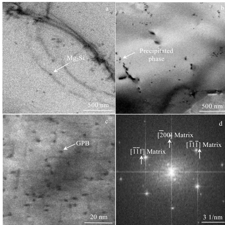
Fig.3 TEM bright field images (a~c) and SAED pattern (d) of B alloy after aging at 175 °C for different time: (a) 0 h, (b) 6 h, and (c, d) 96 h
