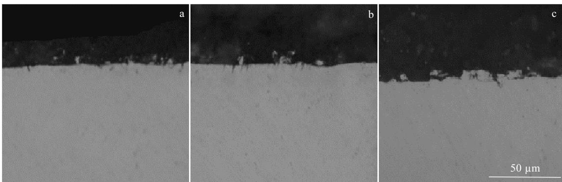
Fig.7 Intergranular corrosion depth of C alloy after aging at 175 °C for 64 h (a), 96 h (b), and 384 h (c)
