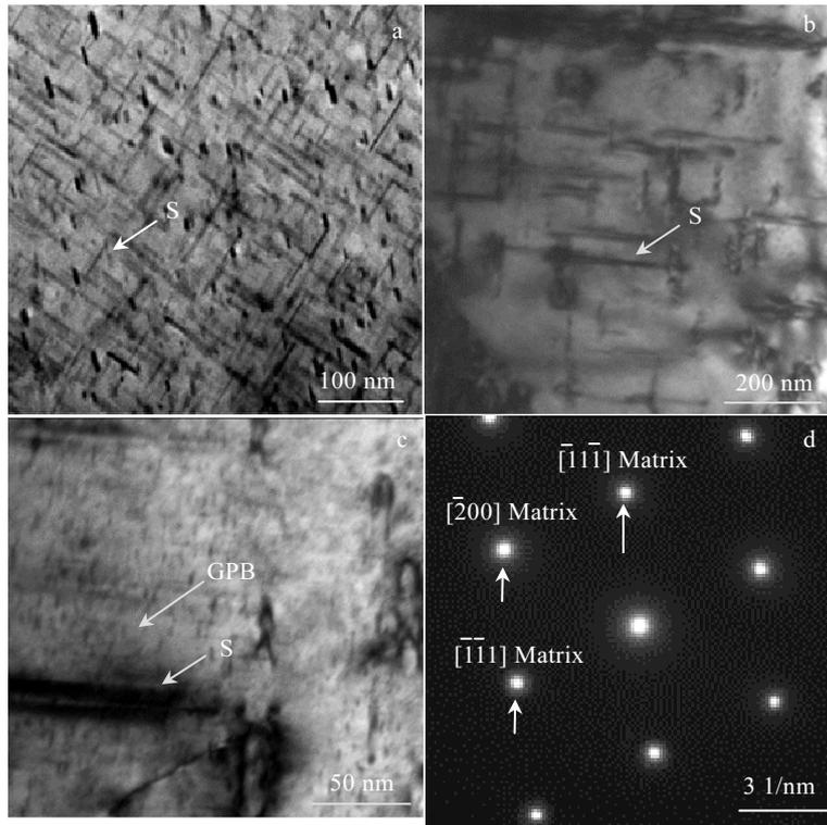
Fig.5 TEM bright field images (a~c) and SAED pattern (d) of D alloy after aging at 175 °C for different time: (a, d) 96 h and (b, c) 240 h
