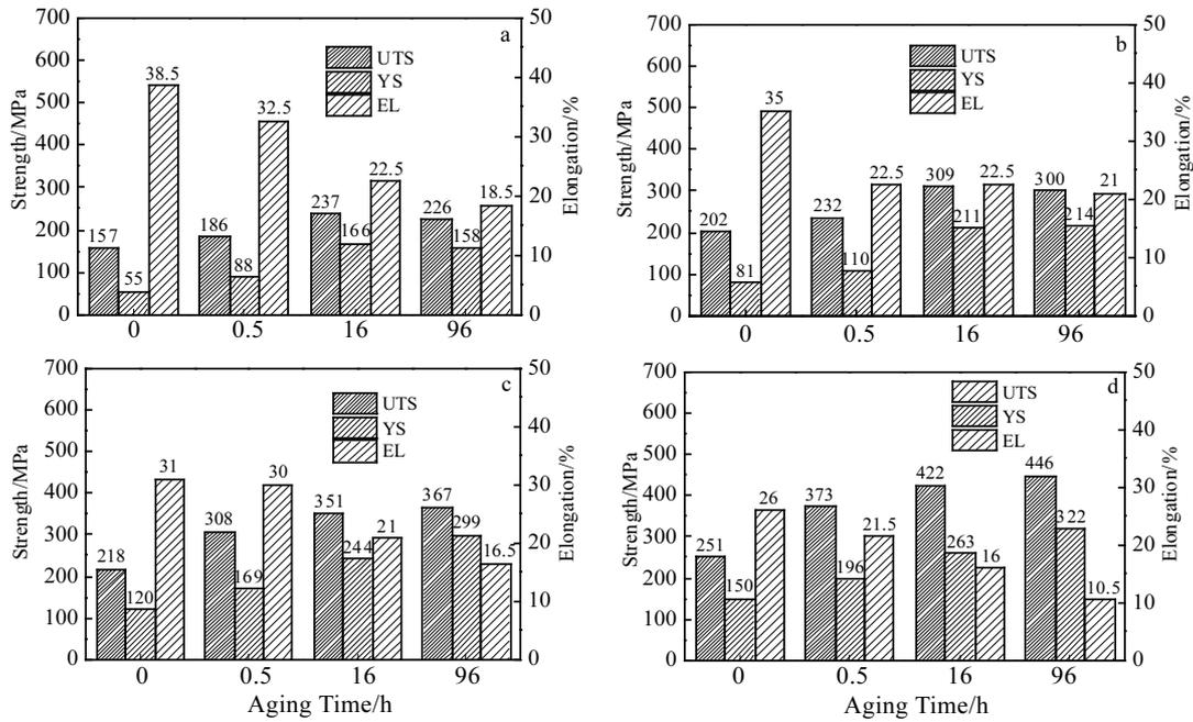
Fig.2 Tensile test results of A (a), B (b), C (c), and D (d) alloys with artificial aging
