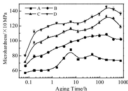
**Fig.1** Microhardness curves of A, B, C and D alloys with isothermal aging at 175 °C after solution treatment at 560 °C for 2 h
