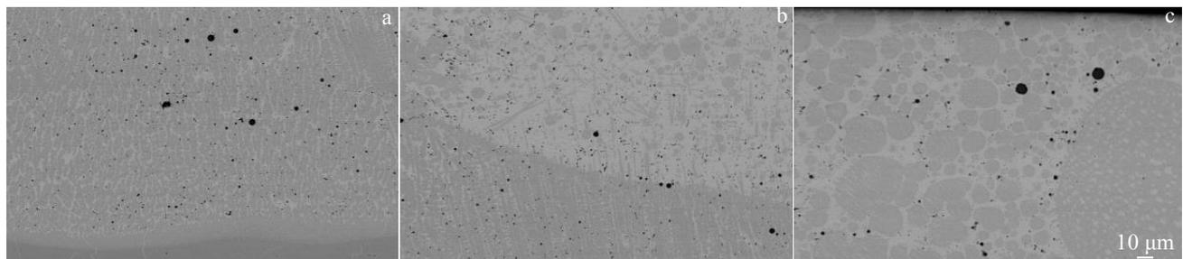
Fig.3 SEM images of cross-section microstructures of bottom (a), middle (b) and top (c) for coating S1
