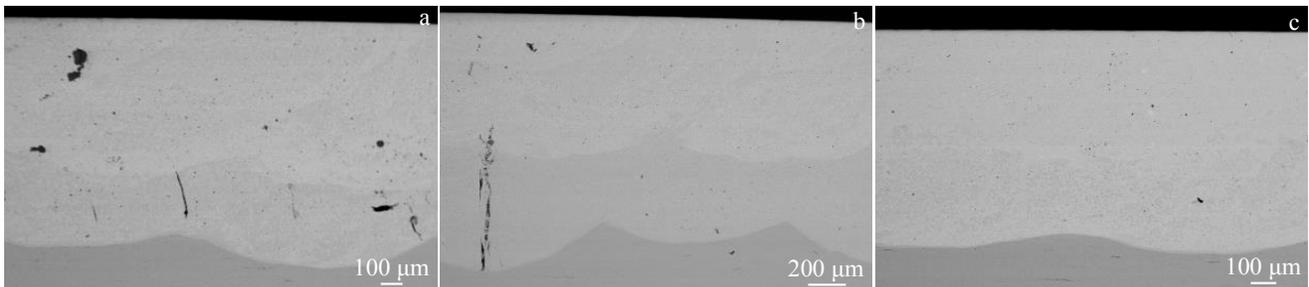
Fig.2 SEM images of cross-section morphology of coatings S1 (a), S2 (b) and S3 (c) at low magnification
