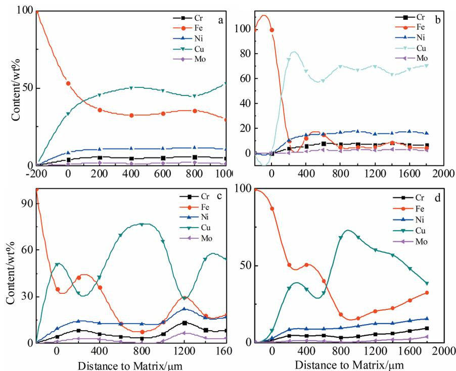
Fig.4 Element content change curves with the distance to matrix for coatings S1 (a), S2 (b), S3 (c), and S4 (d)
