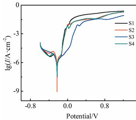
Fig.5 Polarization curves of coatings S1, S2, S3 and S4
