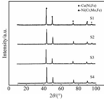
Fig.1 XRD patterns of coatings S1, S2, S3 and S4
