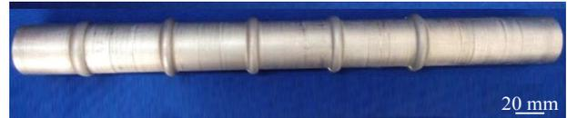
Fig.12 Formed magnesium alloy long axis bellow part
