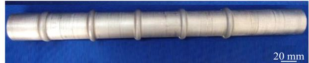
Fig.12 Formed magnesium alloy long axis bellow part
