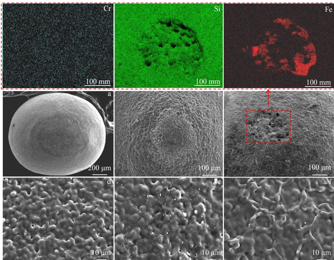
Fig.4 Surface morphologies (a~f) and corresponding EDS mapping of area marked in Fig.4c for  $\text{Li}_4\text{SiO}_4$  pebbles contacted with ODS steel at different temperatures for 300 h: (a, d) 500 °C, (b, e) 600 °C, and (c, f) 700 °C
