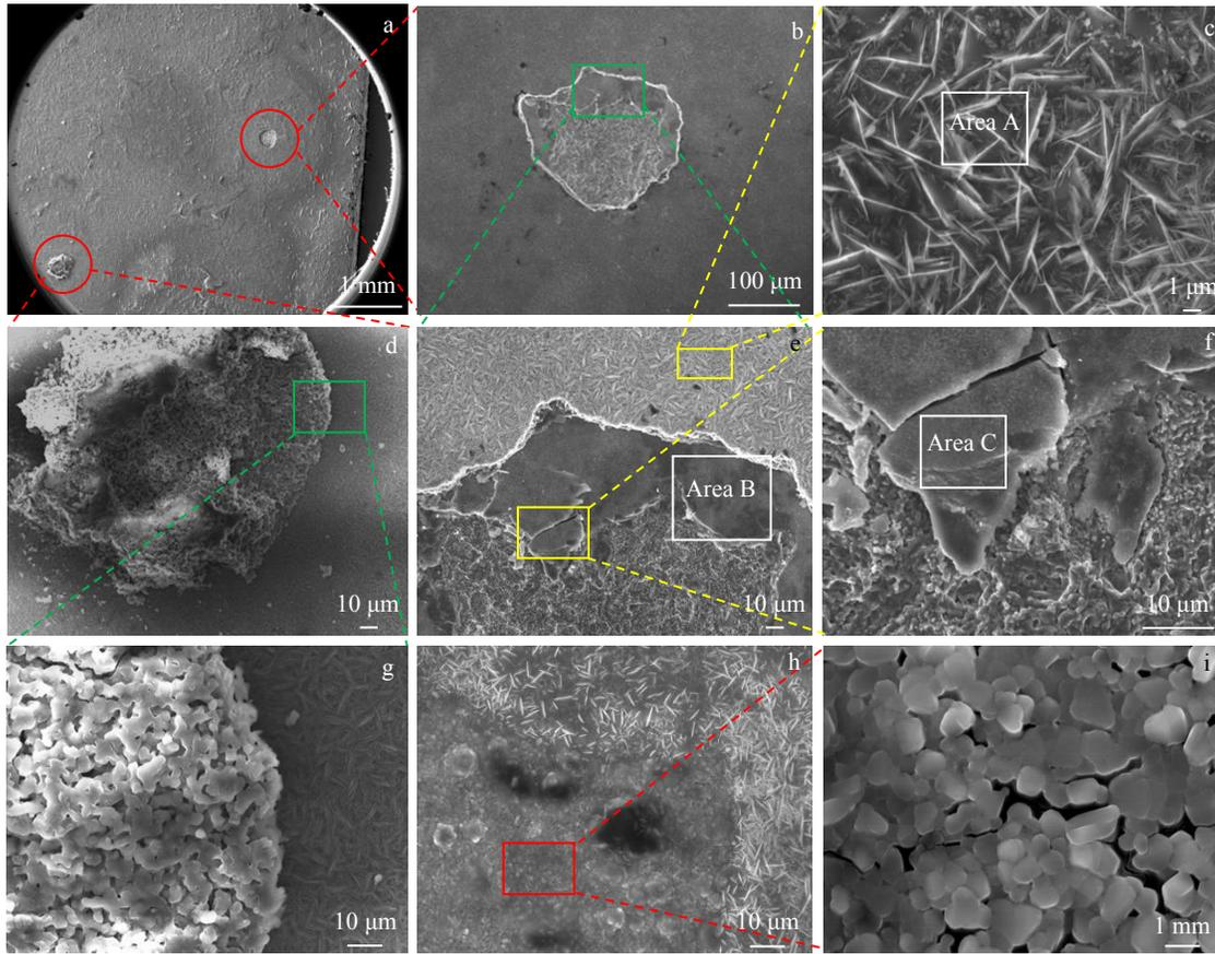
Fig.7 SEM images and EDS analysis areas of ODS steel surface heated with  $\text{Li}_4\text{SiO}_4$  pebbles at 700 °C for 300 h
