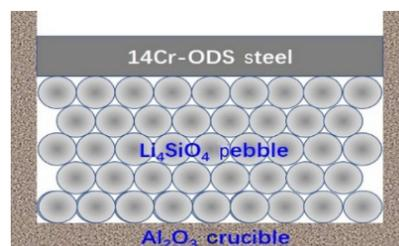
Fig.2 Schematic diagram of loading samples
