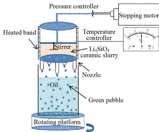
Fig.1 Equipment drawing for preparing  $\text{Li}_4\text{SiO}_4$  pebbles
