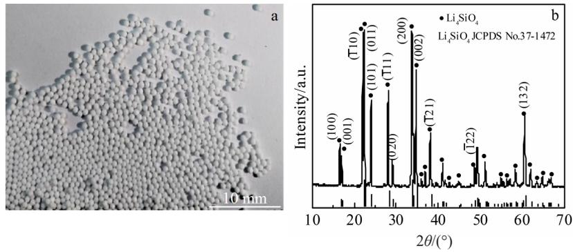
Fig.3 Morphology (a) and XRD patterns (b) of  $\text{Li}_4\text{SiO}_4$  pebbles
