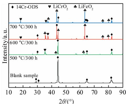
Fig.5 XRD patterns of ODS steel at different heating temperatures
