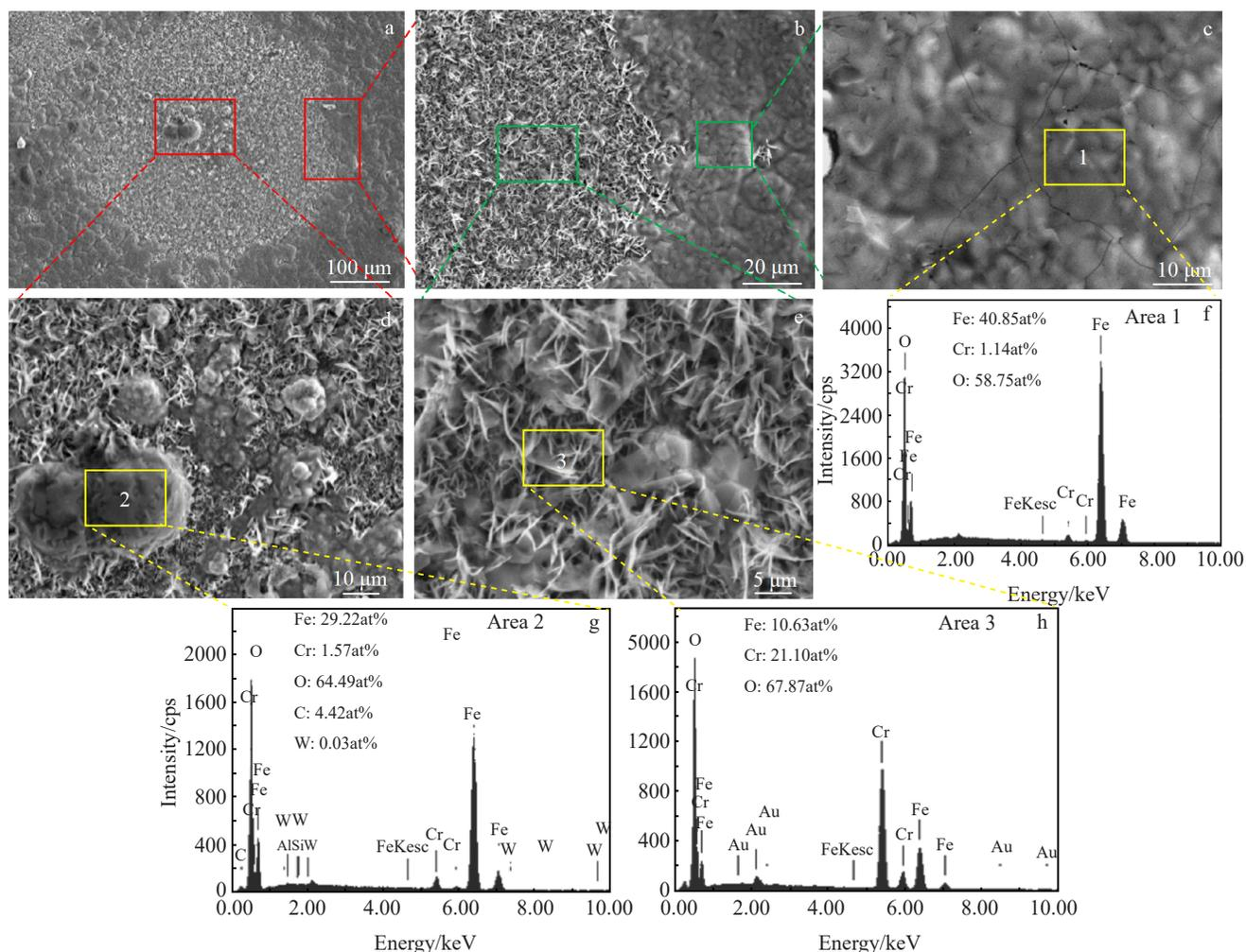
Fig.6 SEM morphologies (a~e) and EDS analysis results of area 1 (f), area 2 (g), and area 3 (h) of ODS steel contacted with  $\text{Li}_4\text{SiO}_4$  pebbles
