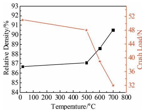
Fig.8 Change of relative density and crush load with temperature for  $\text{Li}_4\text{SiO}_4$  pebbles
