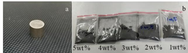
Fig.1 Bonded NdFeB standard cylindrical specimen (a) and magnetic powder after mixing (b)
