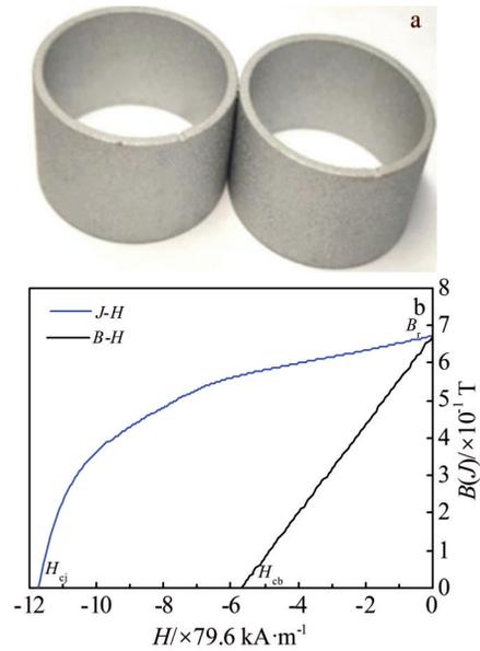
Fig.5 Optical photographs of the ring-shaped magnet (a) and magnetic properties of the RSM (b)
