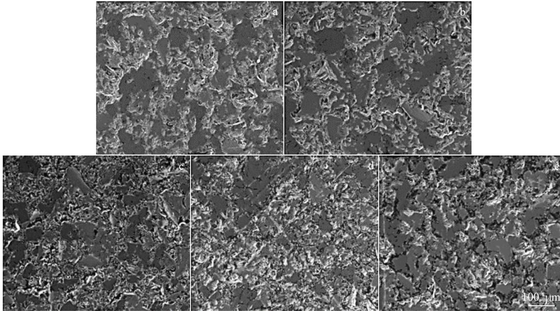
Fig.2 Surface morphologies and structures of bonded magnets with different binder contents: (a) 1wt%, (b) 2wt%, (c) 3wt%, (d) 4wt%, and (e) 5wt%
