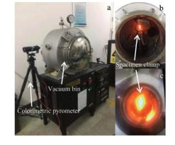
Fig.1 Appearances of thermal shock resistance experiments in vacuum and air: (a) experiment device; (b) thermal shock experiment in air; (c) thermal shock experiment in vacuum
