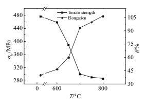
Fig.3 Ultimate tensile strength  $\sigma_b$  and elongation  $\varepsilon$  of Cu-1.04Cr-0.16Zr alloy at different brazing temperatures
