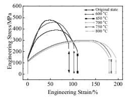
Fig.2 Tensile stress-strain curves of Cu-1.04Cr-0.16Zr alloy at different brazing temperatures
