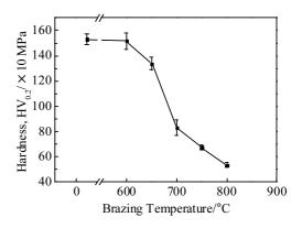
Fig.4 Microhardness of Cu-1.04Cr-0.16Zr alloy at different brazing temperatures
