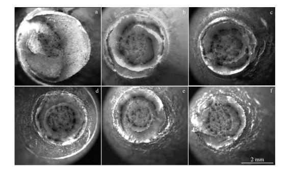
Fig.5 Macroscopic fracture morphologies of Cu-1.04Cr-0.16Zr alloy at different brazing temperatures: (a) original state, (b) 600 °C, (c) 650 °C, (d) 700 °C, (e) 750 °C, and (f) 800 °C
