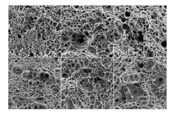
Fig.6 Fracture morphologies of Cu-1.04Cr-0.16Zr alloy at different brazing temperatures: (a) original state, (b) 600 °C, (c) 650 °C, (d) 700 °C, (e) 750 °C, and (f) 800 °C
