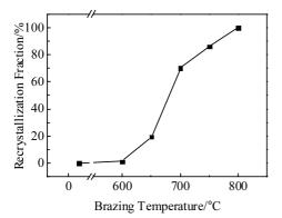
Fig.7 Recrystallization fraction of Cu-1.04Cr-0.16Zr alloy at different brazing temperatures
