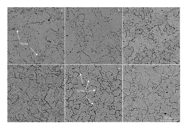
Fig.1 SEM images of Cu-1.04Cr-0.16Zr alloy at different brazing temperatures: (a) original state, (b) 600 °C, (c) 650 °C, (d) 700 °C, (e) 750 °C, and (f) 800 °C
