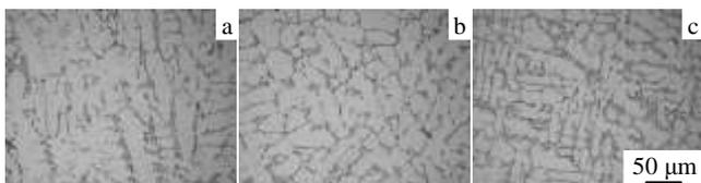
Fig.6 Optical micrographs of the microstructures of surfacing layers welded with wires of different Si contents: (a) 5.0% Si, (b) 5.5% Si, and (c) 5.9% Si
