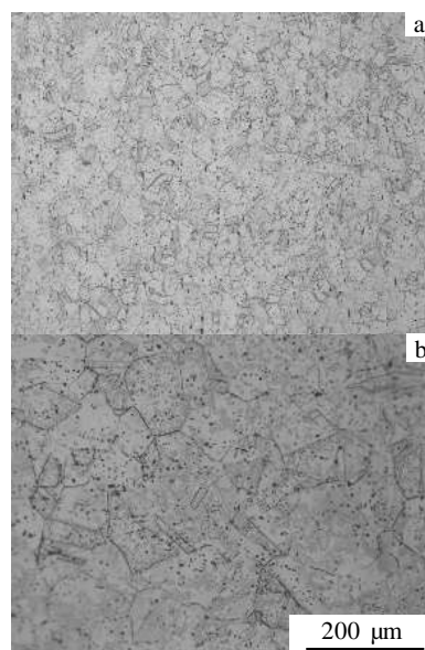
图 1 Ni9.3W 合金均匀化前和均匀化后的截面金相显微组织 Fig.1 Metallographic microstructure of Ni9.3W alloy: (a) before the homogenization and (b) after the homogenization
