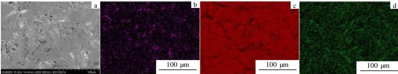
Fig.4 SEM image (a) and EDS map of the sample with Ni (3wt%) after sintering: (b) Ni, (c) W, and (d) C
