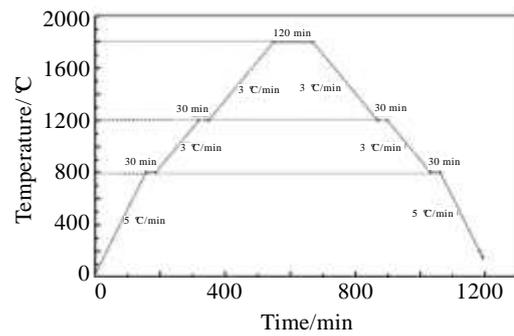
Fig.2 Sintering temperature and holding time of liquid phase sintering (LPS)
