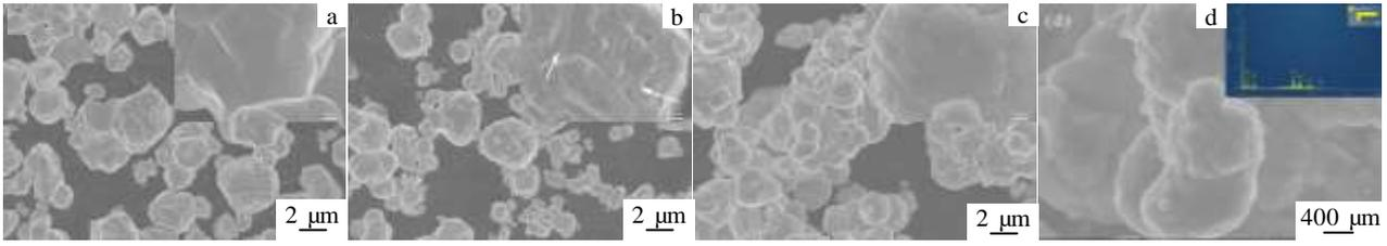
Fig.3 Surface morphologies image of the WC powder: (a) original WC powder, (b) pretreated WC powders, (c) WC powders after electroless Ni plating, and (d) high magnification image of Fig.3c coupled with EDS
