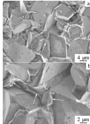
Fig.8 Surface morphology of fractured WC-Ni composite
