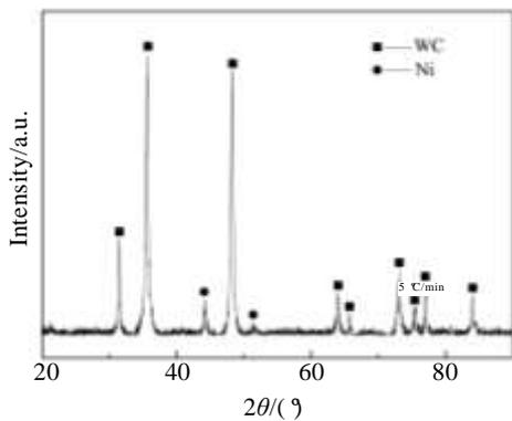
Fig.5 XRD pattern of the WC-9wt% Ni composites
