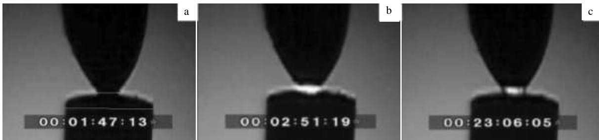
Fig.6 Observation on the behavior of molten bridge under direct current 6 V, 15 A: (a) stable molten bridge with approximate cylindrical shape, (b) large amounts arc, and (c) clear arc in the middle ( v=50.0 mm/s, f=50.0 cN, N=480 fps)
