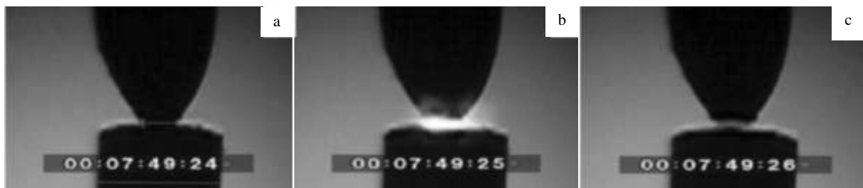
Fig.8 Observation on the behavior of molten bridges under direct current 6 V, 20 A: (a) a molten bridge, (b) great deals of arc, and (c) the contact pair are in complete separation and the molten bridge and arc ( v=50.0 mm/s, f=50.0 cN, N=480 fps)
