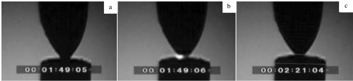
Fig.5 Observation on the behavior of molten bridges under direct current 6 V, 12 A: (a) approximate dumbbell shaped molten bridge, (b) molten bridge break (obvious arc appears on the left), and (c) approximate cylindrical molten bridge ( v=50.0 mm/s, f=50.0 cN, N=480 fps)
