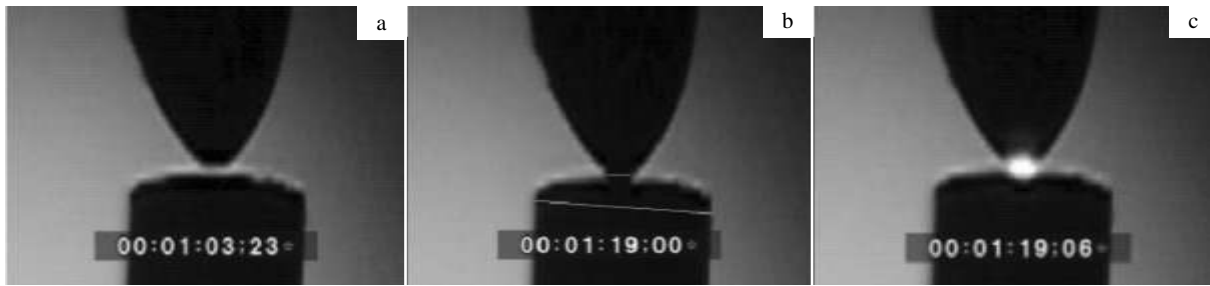
Fig. 3 Observation on the behavior of molten bridges under direct current 6 V, 8 A: (a) without contact, (b) stable molten bridge, and (c) palpable arc ( v=50.0 mm/s, f=50.0 cN, N=480 fps)
