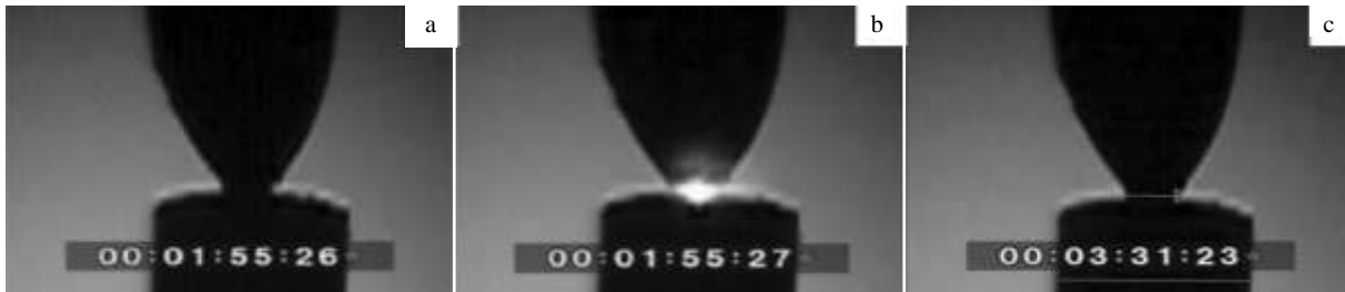
Fig.7 Observation on the behavior of molten bridges under direct current 6 V, 18 A: (a) approximate dumbbell shaped molten bridge, (b) dazzling arc, and (c) stable molten bridge with approximate cylindrical shape ( v=50.0 mm/s, f=50.0 cN, N=480 fps)
