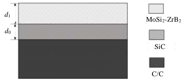
Fig.1 Schematic of the SiC/MoSi 2 -ZrB 2 coating structure
