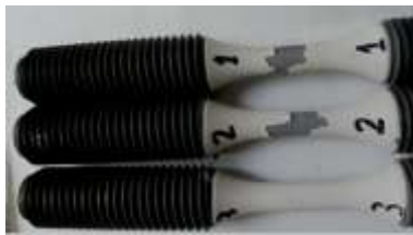
Fig.4 Spallation of TBC systems (1- \Delta\varepsilon=-0.45\% , OP; 2- \Delta\varepsilon=-0.30\% , OP; 3- \Delta\varepsilon=0.30\% , IP)
