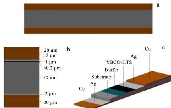
Fig.2 Schematic view of the studied YBCO CC tape (Super Power SCS4050)
