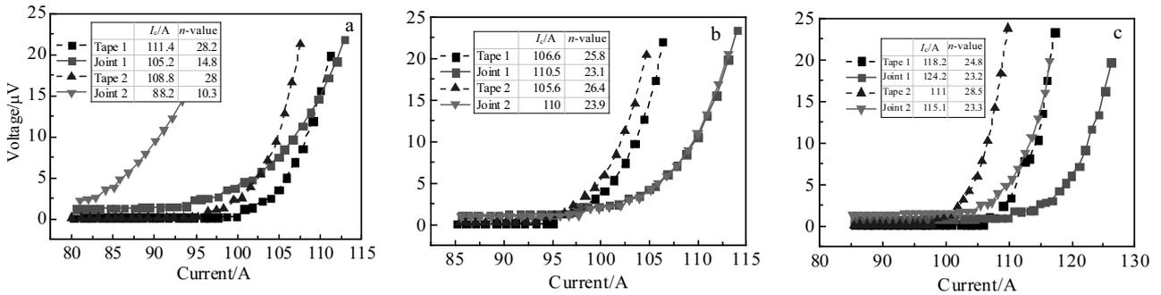
Fig.6 Characteristic curves of the pristine tape and corresponding joint, representing by dash and solid, respectively: (a) 5 cm-long joints, (b) 8 cm-long joints, and (c) 11 cm-long joints
