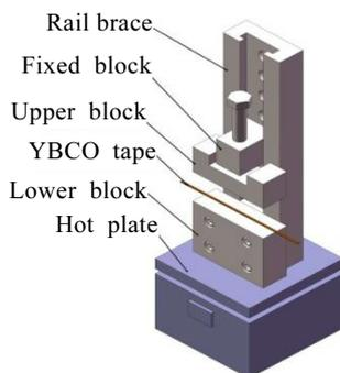
Fig.3 Three-dimensional model of the lapped joints soldering device having a high smooth interface of the upper block and lower block
