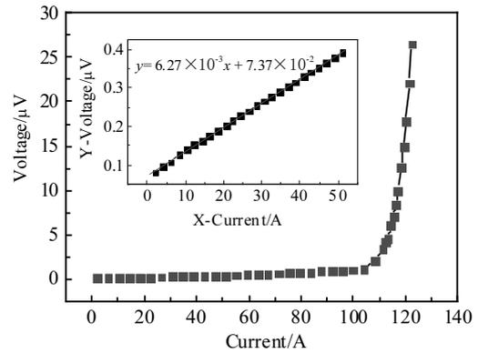
Fig.5  $V$ - $I$  characteristic curve for the sample with length of 14 cm and thickness less than 10  $\mu\text{m}$
