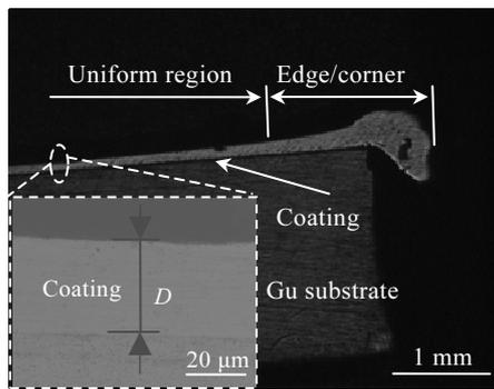
Fig.6 Measurement direction of electrodepositing coating thickness
