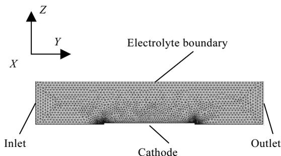
Fig.1 YZ section of electrodeposition physical model when  $X=25$  mm
