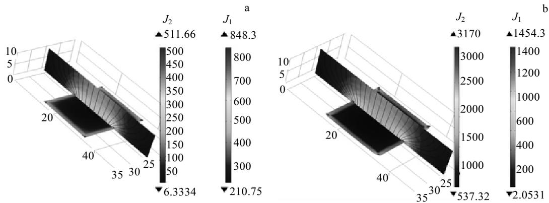
Fig.2 Current density distribution of electrodepositing system: (a)  $J = 300 \text{ A/m}^2$  and (b)  $J = 900 \text{ A/m}^2$
