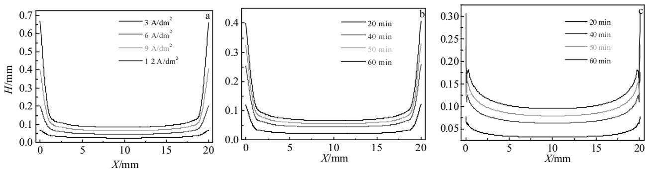
Fig.3 Simulative thickness in the center of the cathode plate: (a) SCF-CO<sub>2</sub>,  $t = 60 \text{ min}$ ; (b) SCF-CO<sub>2</sub>,  $J = 9 \text{ A/dm}^2$ ; (c) general environment,  $J = 9 \text{ A/dm}^2$
