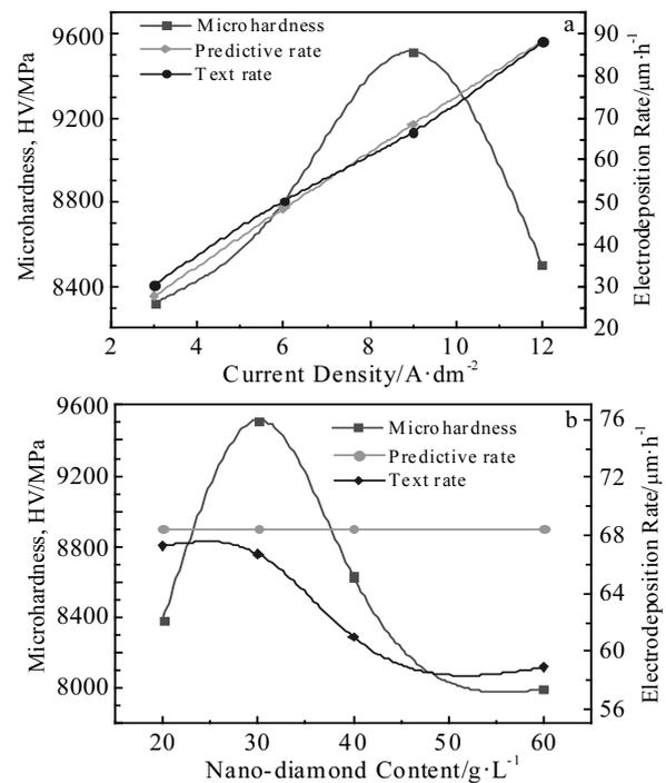
Fig.7 Effects of current density (a) and nano-diamond content (b) on micro-hardness, electrodeposition rate, and text rate
