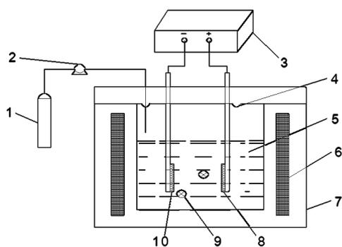
1-CO<sub>2</sub> cylinder; 2-high-pressure pump; 3-power supply; 4-vent; 5-electrolyte solution; 6-thermostatic bath; 7-reactor; 8-anode; 9-mechanical agitator; 10-cathode
