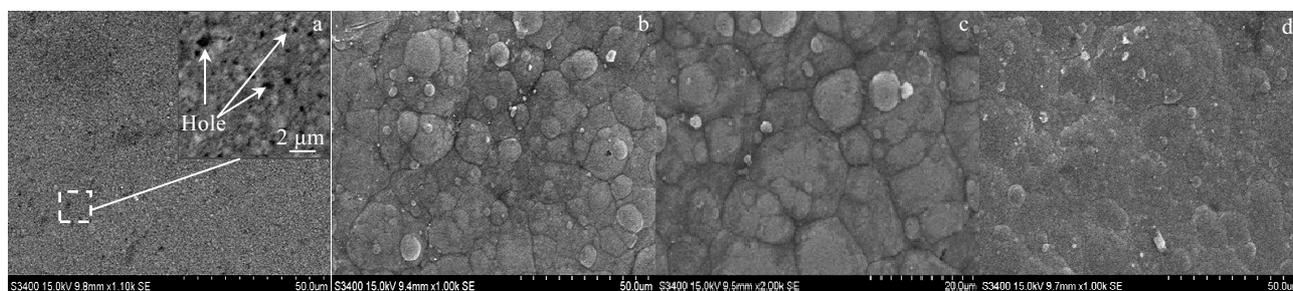
Fig.5 Ni-diamond electrodepositing coating morphologies under different conditions: (a) general conditions; SCF-CO<sub>2</sub> conditions: (b) 0.24 A, 3 g; (c, d) 0.36 A, 3 g
