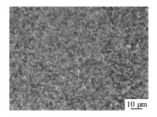
Fig.1 Original microstructure of alloy billet
