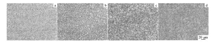
Fig.2 Morphologies of primary  $\alpha$  phase after different solution treatments: (a) specimen 1, (b) specimen 2, (c) specimen 3, and (d) specimen 4
