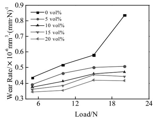
Fig.1 Wear rate of Ti6Al4V alloy and composites as a function of load
