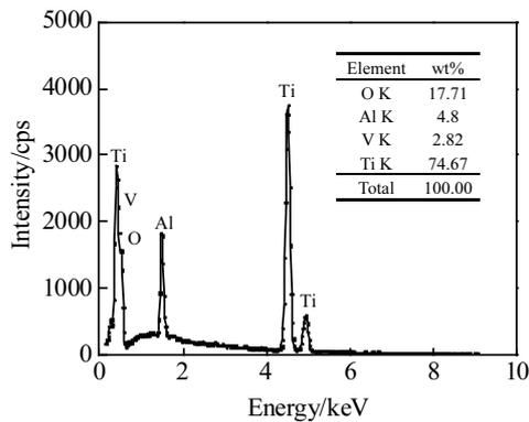
Fig.9 EDS analysis of the wear debris in Fig.8a
