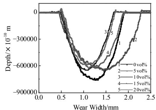
Fig.3 Wear depth of Ti6Al4V alloy and composites with different volume fractions of reinforcing phases under 15 N
