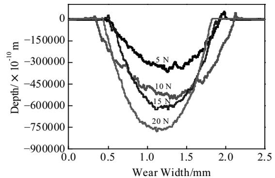
Fig.2 Wear depth of composites with volume fraction of 15% as a function of load
