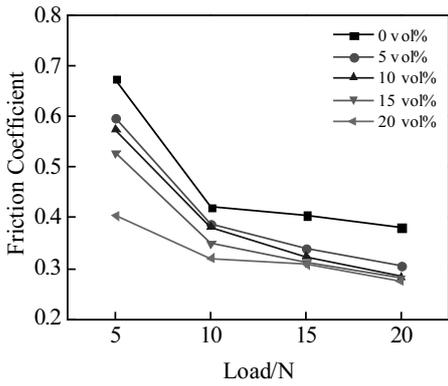
Fig.4 Variation of the friction coefficient for the Ti6Al4V alloy and composites under different loads
