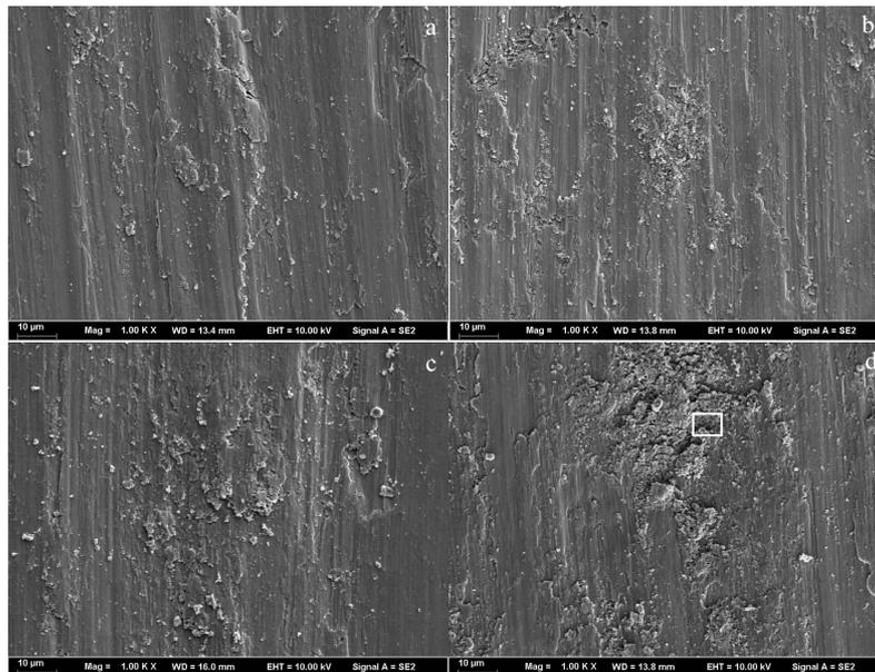
Fig.6 Worn surface morphologies of (TiC+TiB)/Ti6Al4V composites with volume fraction of 15% under different loads: (a) 5 N, (b) 10 N, (c) 15 N and (d) 20 N
