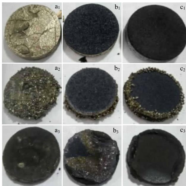
Fig.3 Morphologies of the Inconel 600 alloy (a), Mo coatings (b), and Al-Mo coatings (c) under different high temperature sulfidation conditions: (a<sub>1</sub>, b<sub>1</sub>, c<sub>1</sub>) 973 K/12 h, (a<sub>2</sub>, b<sub>2</sub>, c<sub>2</sub>) 1073 K/12 h, (a<sub>3</sub>, c<sub>3</sub>) 1173 K/12 h, (b<sub>3</sub>) 1173 K/8 h
