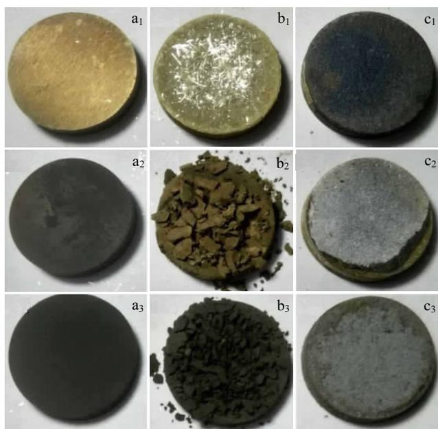
Fig.7 Morphologies of Inconel 600 (a), Mo coatings (b) and Al-Mo coatings (c) under different high-temperature oxidation conditions: (a<sub>1</sub>,b<sub>1</sub>,c<sub>1</sub>) 973 K/12 h, (a<sub>2</sub>,b<sub>2</sub>,c<sub>2</sub>) 1073 K/8 h, (a<sub>3</sub>,b<sub>3</sub>,c<sub>3</sub>) 1173 K/2 h
