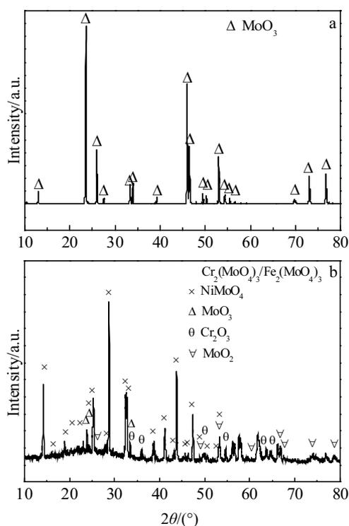
Fig.8 XRD patterns of Mo coatings after oxidation at 973 K for 12 h (a) and 1173 K for 2 h (b)
