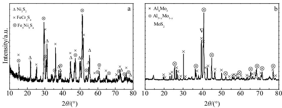
Fig.5 XRD patterns of Inconel 600 alloy after sulfidation at 1073 K for 8 h (a) and Al-Mo coating with a Mo bonding layer after sulfidation at 1173 K for 109 h (b)
