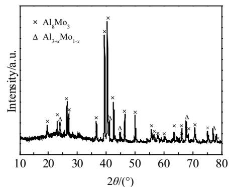
Fig.1 XRD pattern of the Al-27at%Mo powders milled for 31 h and heat treated at 1273 K for 2 h
