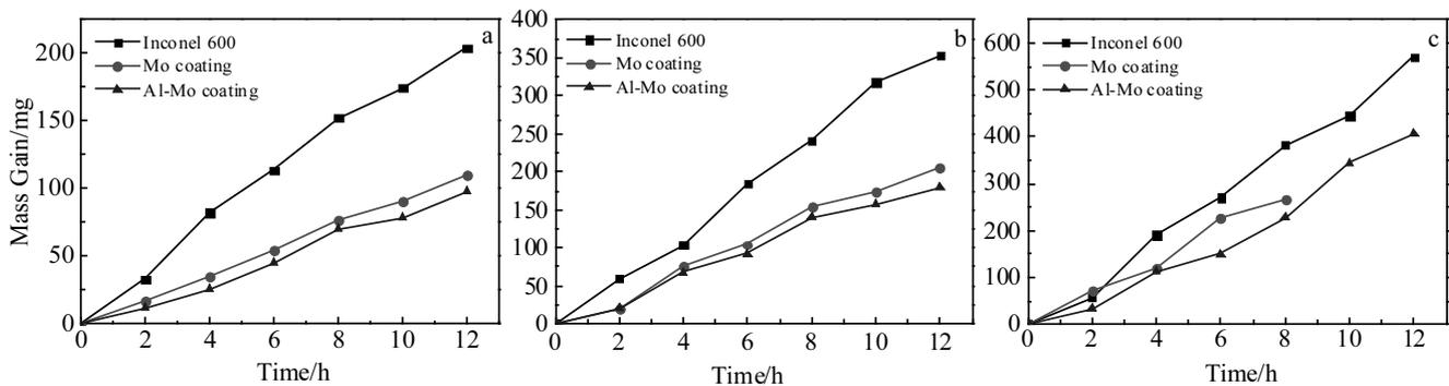
Fig.6 Mass gain of Al-Mo coatings, Mo coatings and Inconel 600 alloy with a Mo bonding layer at 973 K (a), 1073 K (b) and 1173 K (c) after the sulfidation
