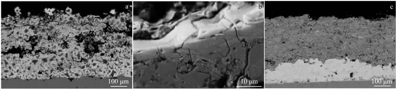
Fig.4 Microstructures of Al-Mo and Mo coatings after sulfidation: (a, b) Mo coating at 973 K/12 h and (c) Al-Mo coating at 1173 K/109 h
