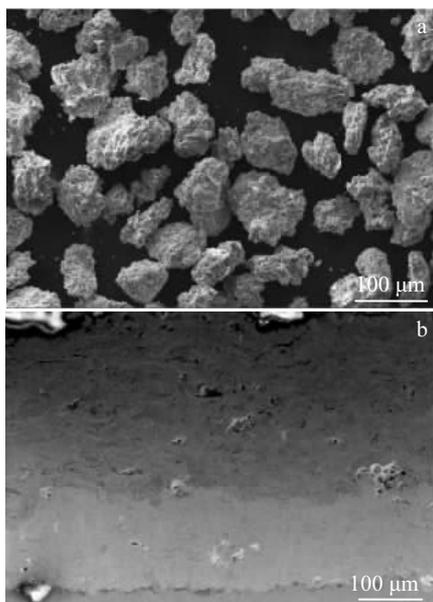
Fig.2 Microstructures of Al-Mo powders (a) and plasma sprayed Al-Mo coatings (b)
