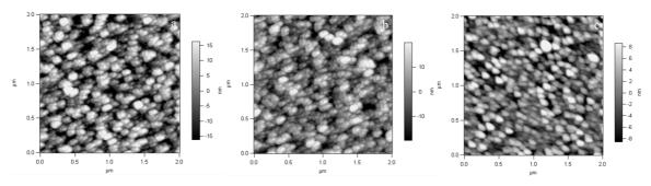
Fig.2 Surface morphologies of La<sub>1-x</sub>Ce<sub>x</sub>MnO<sub>3</sub> thin films: (a) x=0.10, (b) x=0.20, and (c) x=0.33
