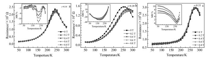
Fig.5 *R-T* curves and magnetic-resistance (MR) versus temperature curves (inset) under the external magnetic field of 0, 0.2, 0.4, 0.6, 0.8 T for the different doping ratios in La<sub>1-x</sub>Ce<sub>x</sub>MnO<sub>3</sub> thin films: (a) *x*=0.10, (b) *x*=0.20, and (c) *x*=0.33
