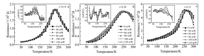
Fig.4 Photo induced resistances as a function of temperature with the light intensity of 0, 40, 60, 80, 100 and 120 mW for the different doping ratios in La<sub>1-x</sub>Ce<sub>x</sub>MnO<sub>3</sub> thin films: (a) x=0.10, (b) x=0.20, and (c) x=0.33
