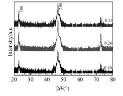
Fig.1 XRD patterns of La<sub>x</sub>Ce<sub>1-x</sub>MnO<sub>3</sub>(LCeMO)/SrTiO<sub>3</sub>(STO)
