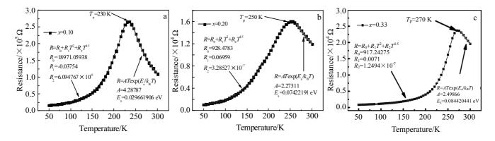
Fig.3 Resistance-temperature (*R-T*) curves and fitting analysis for the different doping ratios in La<sub>1-x</sub>Ce<sub>x</sub>MnO<sub>3</sub> thin films: (a) x=0.10, (b) x=0.20, and (c) x=0.33
