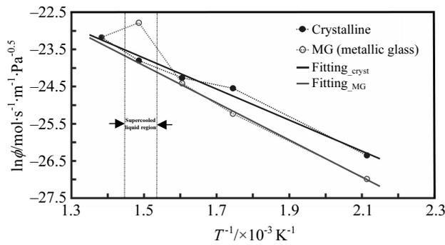
Fig.4 Arrhenius plots of the hydrogen permeation rates  $\phi$
