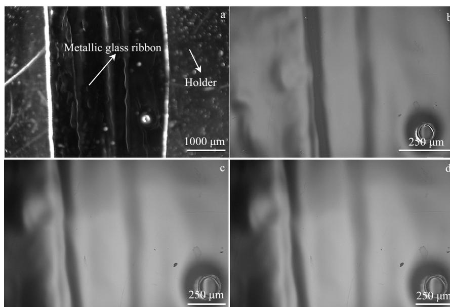
Fig.3 Optical images of Pd<sub>71.5</sub>Cu<sub>12</sub>Si<sub>16.5</sub> metallic glass ribbon during the hydrogen absorption and desorption cycles: (a) initial ribbon, (b) after 2 cycles, (c) after 10 cycles, and (d) after 10 cycles and immersed in H<sub>2</sub> atmosphere for 16 h
