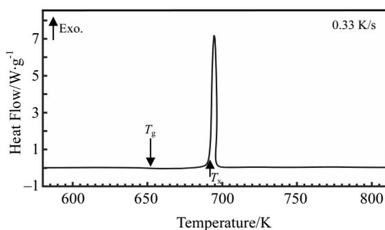
Fig.2 DSC curve of the Pd<sub>71.5</sub>Cu<sub>12</sub>Si<sub>16.5</sub> metallic glass ribbon
