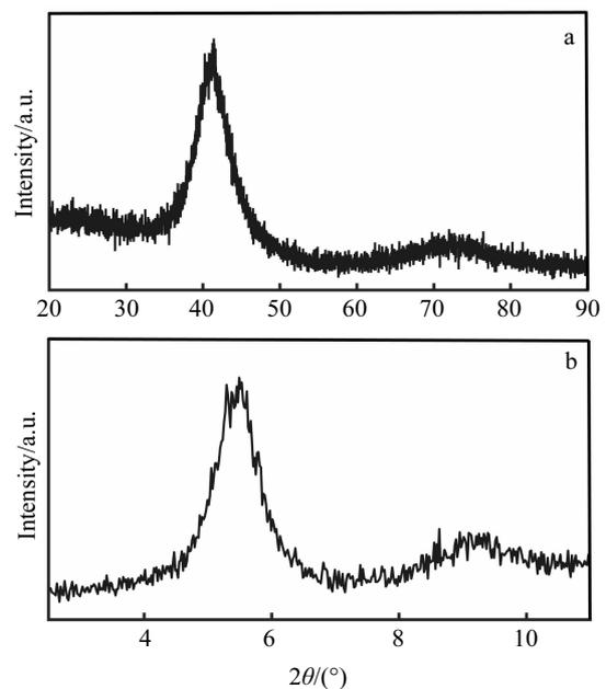
Fig.1 Structural analysis of Pd<sub>71.5</sub>Cu<sub>12</sub>Si<sub>16.5</sub> metallic glass ribbons obtained by the conventional XRD (a) and short wavelength X-ray stress analyzer (b)
