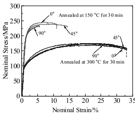
Fig.2 Nominal stress-strain curves in the tensile direction of RD, 45°, and TD of the sheets annealed at 150 and 300 °C for 30 min
