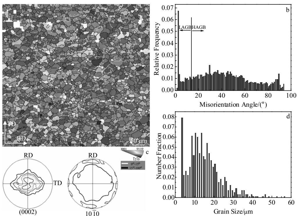
Fig.3 Inverse pole figure (IPF) map with horizontal RD (a), misorientation distribution profile (b), pole figure (c) and grain size distribution (d) of the sheet annealed at 300 °C for 30 min
