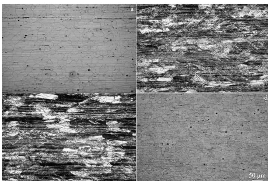
Fig.1 Optical microstructures of the sheet taken in the longitudinal section with horizontal ND/RD: (a) as-extruded condition, (b) as-rolled condition, and the same sheet rolled and annealed at 150 °C (c) and 300 °C (d) for 30 min
