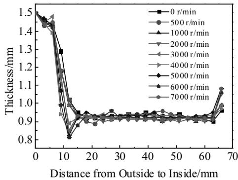
Fig.9 Thickness distribution of parts formed at different rotation speeds
