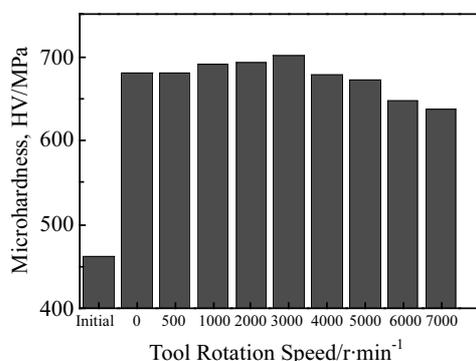
Fig.7 Micro-hardness values of AA7075-O formed parts at various rotation speeds
