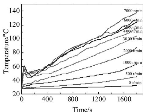
Fig.6 Temperature trends of AA7075-O sheets at different tool rotation speeds
