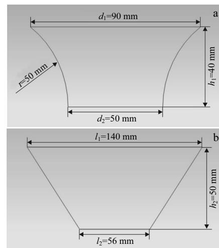
Fig.1 Geometrical details of designed parts: (a) truncated funnel and (b) pyramid frustum
