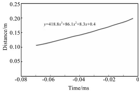
Fig.4 Distance-time curve of the detonation wave
