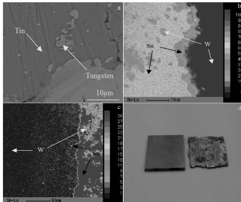
Fig.1 SEM microstructures of the diffusion-bonded joint (a); Sn mapping of interface zone for the cross-section specimens sintered at 600 °C (b) and 800 °C (c) by EPMA; unsintered and sintered (800 °C) specimens (d)
