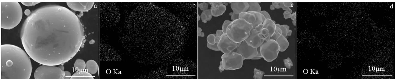
Fig.5 SEM image of tin particles (a); O mapping of tin particles (b); SEM image of tungsten particles (c); O mapping of tungsten particles (d)
