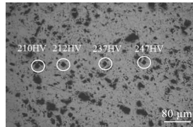
Fig.10 Variations of microhardness of the specimen
