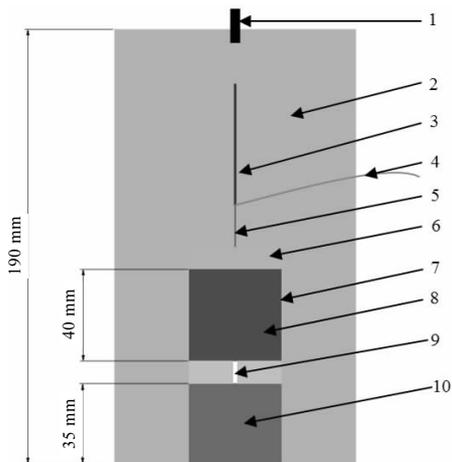
1 detonator; 2 explosive; 3 continuous velocity probe; 4 wire; 5 support structure of continuous velocity probe; 6 steel; 7 steel tube; 8 tungsten-tin alloy particles; 9 venthole; 10 steel block
