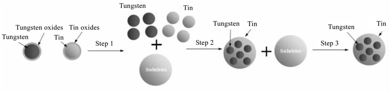
Fig.2 Schematic of the encapsulating process
