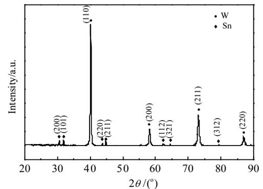
Fig.6 XRD pattern of tungsten-tin composite powder sintered at 300 °C with alkaline solution
