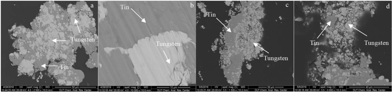
Fig.7 SEM images of specimen sintered at 300 °C with alkaline solution (a, b) and at 800 °C without alkaline solution (c, d)
