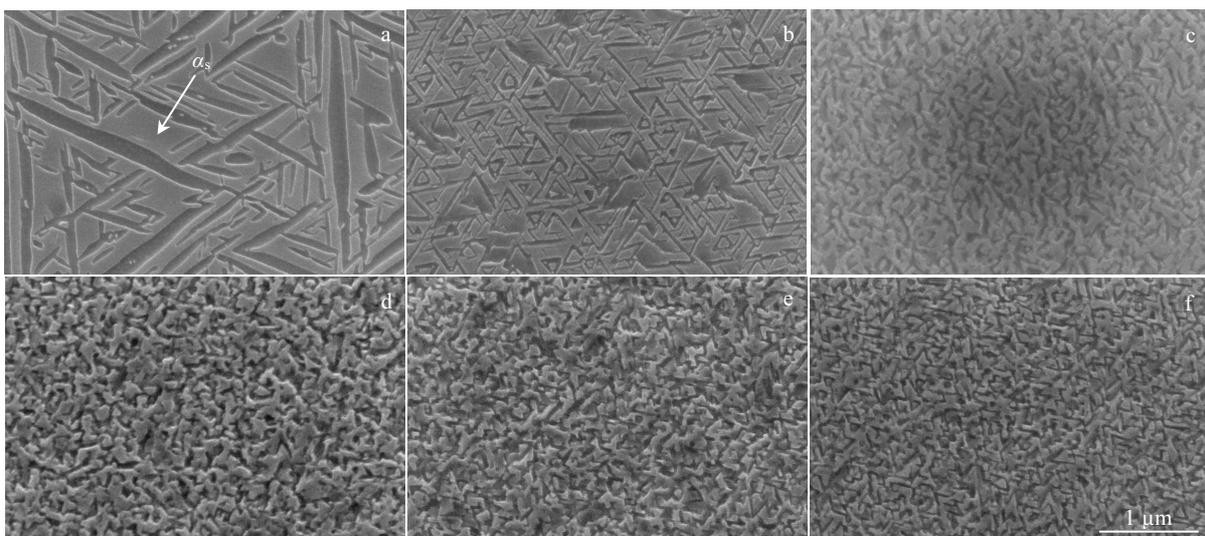
Fig.4 Comparison of microstructures between SA and DA conditions: (a) 550 °C/4 h; (b) 350 °C/5 min+550 °C/4 h; (c) 350 °C/0.5 h+550 °C/4 h; (d) 350 °C/2 h+550 °C/4 h; (e) 350 °C/4 h+550 °C/4 h; (f) 350 °C/8 h+550 °C/4 h
