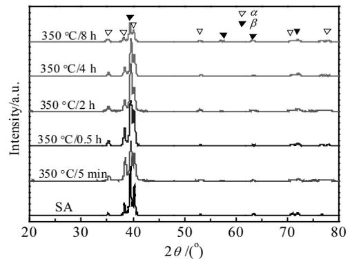
Fig.3 XRD patterns of the alloy under SA and DA conditions
