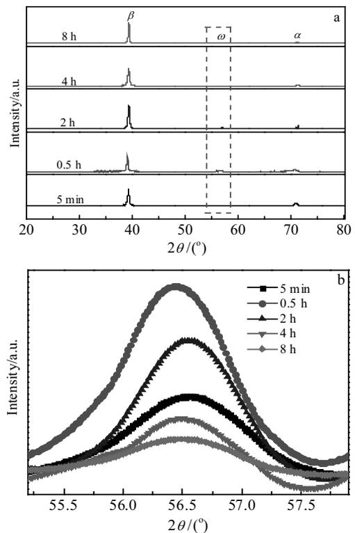
Fig.2 XRD patterns of PA conditions: (a) the diffraction peaks of  $\beta$ ,  $\alpha$  and  $\omega$  phases; (b) the diffraction peaks of  $\omega$  phase
