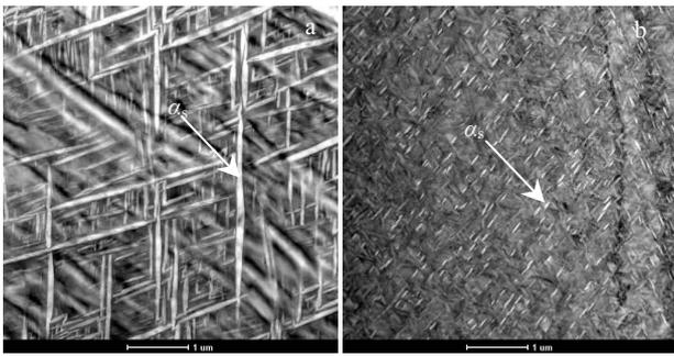
Fig.5 STEM images of DA conditions: (a) PA for 0.5 h and (b) PA for 2 h
