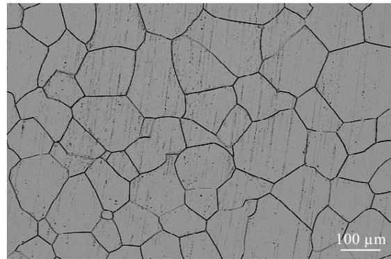
Fig.1 Metallurgical microstructure of the alloy solution treated at 830 °C
