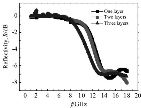
Fig.11 Effect of layer number on reflectivity of composite materials
