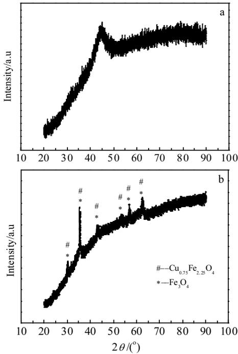
Fig.6 XRD patterns of strips before (a) and after (b) modification
