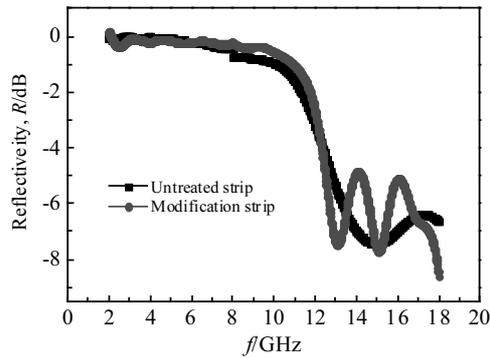
Fig.10 Reflectivity of composite materials
