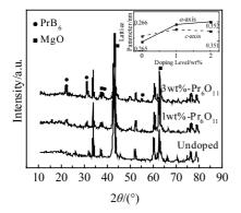
Fig.1 XRD patterns of the Pr<sub>6</sub>O<sub>11</sub>-doped MgB<sub>2</sub> samples after heating at 850 °C for 24 h (Inset: *a*, *c*-axis lattice parameters of MgB<sub>2</sub>)
