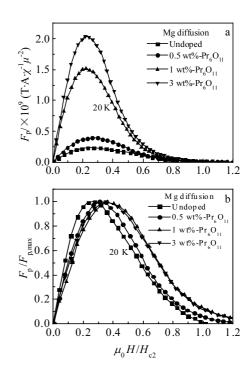
Fig.5 Flux pinning force as a function of applied magnetic field at 20 K: (a) flux pinning force  $F_p$  and (b) normalized flux pinning force  $F_p/F_{p,max}$
