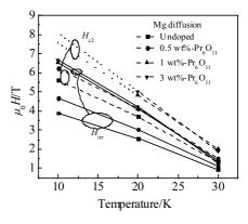
Fig.4 Temperature dependence of the irreversibility field  $H_{irr}$  and upper critical field  $H_{c2}$
