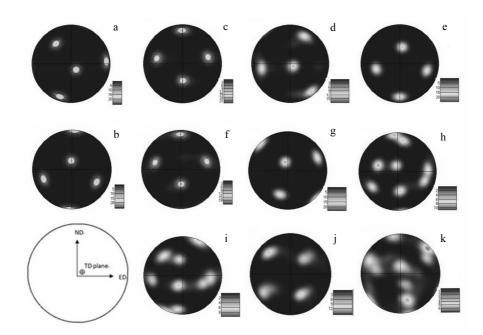
Fig.5 {111} pole figures of samples after ECAP for several passes by route A, Bc and C: (a) initial condition; (b) 1 pass; (c) 2 passes of route A;
