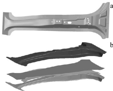
Fig.3 Geometry (a) and FE model (b) of B pillar
