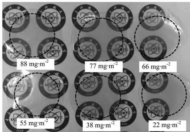
Fig.3 Photos of AgNWs/rGO films with 220  $\text{mg}\cdot\text{m}^{-2}$  AgNWs and different deposition densities of rGO
