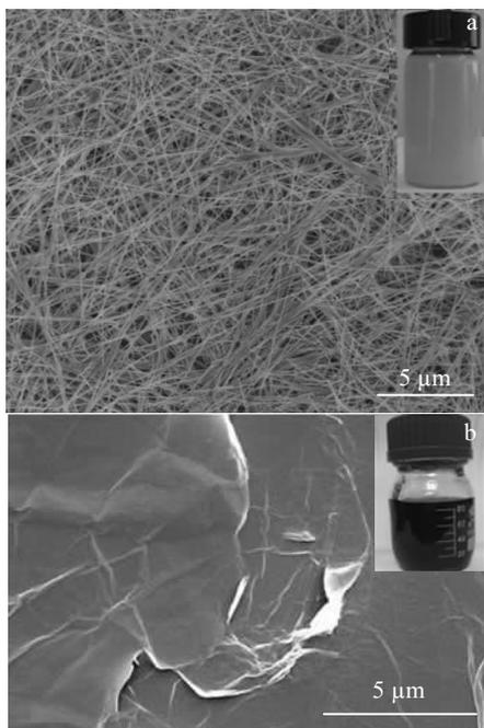
Fig.2 SEM images of AgNWs (a) and rGO (b); inserts are photos of AgNWs and rGO synthesized
