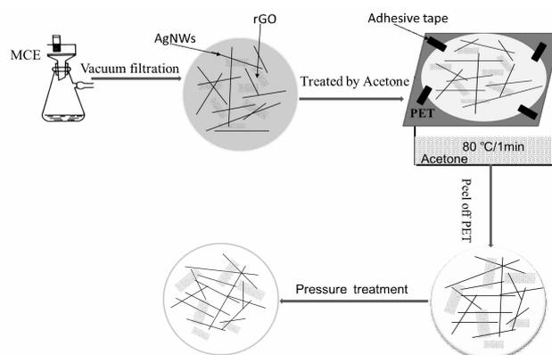
Fig.1 Schematic of fabrication process of AgNWs/rGO-MCE film
