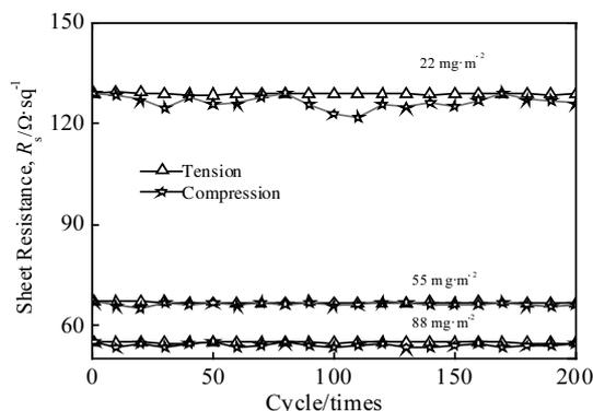
Fig.8  $R_s$  of AgNWs-rGO films after cycles of folding up
