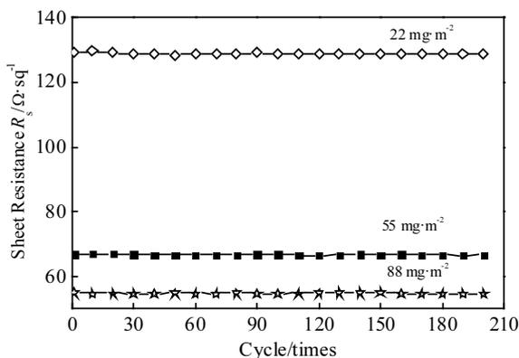
Fig.7  $R_s$  of AgNWs-rGO films after taping test
