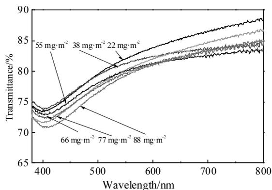
Fig.4 Optical transmittance spectra of AgNWs-rGO films with different rGO deposition densities
