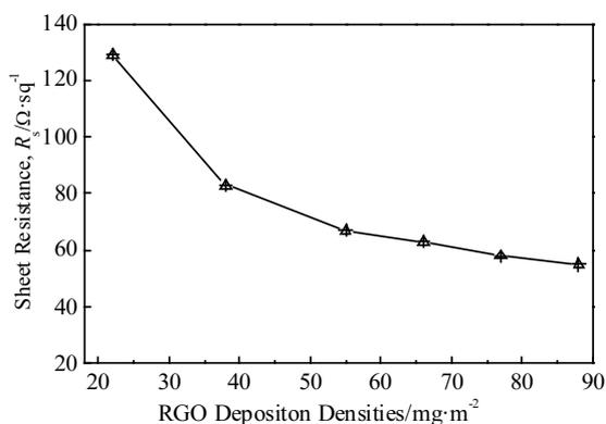
Fig.6  $R_s$  versus rGO deposition density of AgNWs/rGO films
