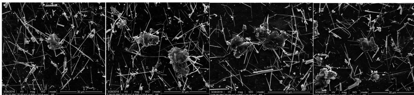
Fig.5 SEM images of AgNWs/rGO films with different rGO deposition densities: (a) 22  $\text{mg}\cdot\text{m}^{-2}$ , (b) 38  $\text{mg}\cdot\text{m}^{-2}$ , (c) 55  $\text{mg}\cdot\text{m}^{-2}$ , and (d) 77  $\text{mg}\cdot\text{m}^{-2}$
