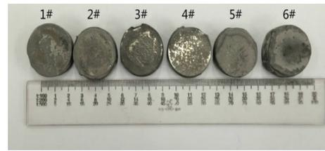
Fig.2 TiAl-based alloy VHPS samples under different conditions described in Table 1
