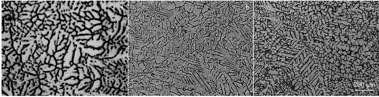
Fig.1 Optical microstructures of the as-cast magnesium alloys: (a) ZM21, (b) ZM21-0.8Y, and (c) ZM21-2.2Y
