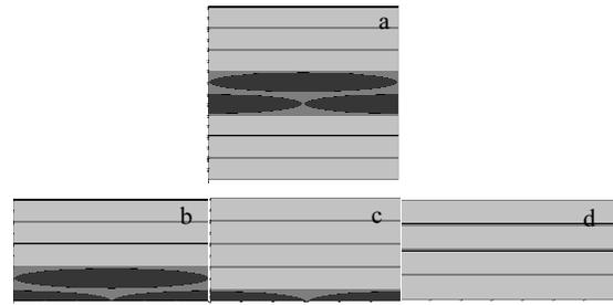
Fig.6 Structural unit cell models for predicting Young's modulus of Cf/AZ91D laminates in different layup modes: (a) L3-2-3, (b) L3-3-3, (c) L4-1-4, and (d) L0-9-0
