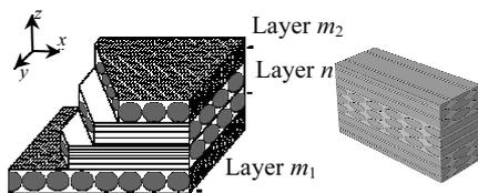
Fig.3 Layup configuration for C<sub>f</sub>/AZ91D laminates
