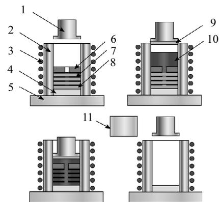
1-punch; 2-container of die; 3-preheating furnace of die; 4-pad; 5-heel block; 6-mould component; 7-graphite sheet; 8-preform; 9-sealing module; 10-liquid magnesium alloy; 11- $C_f/AZ91D$  laminates
