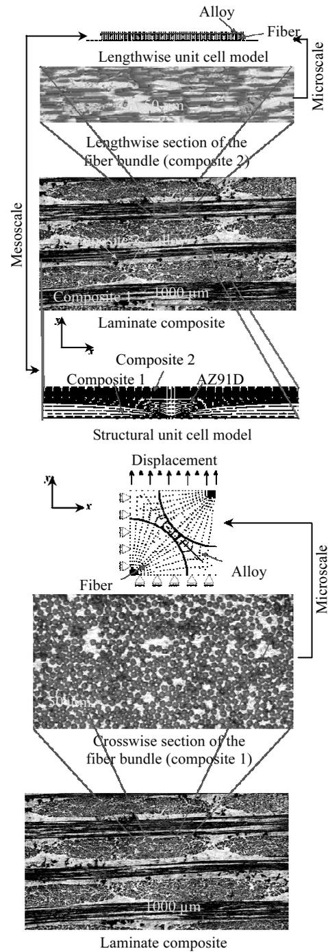
Fig.5 Detailed schematic diagram of multi-scale modeling for C<sub>f</sub>/AZ91D laminates
