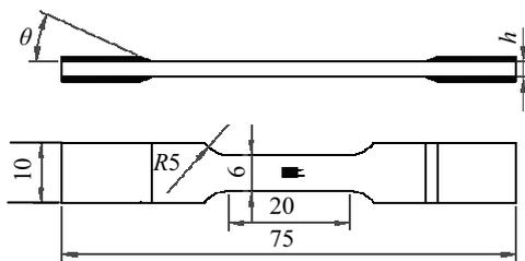
Fig.4 Dimension for tensile test specimen ( $h$  is specimen's thickness,  $h=2\sim 3$  mm;  $\theta$  is strengthening plate chamfering,  $\theta\geq 15^\circ$ )
