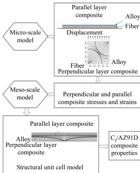
Fig.1 Schematic diagram for multi-scale analysis of  $C_f/AZ91D$  laminates
