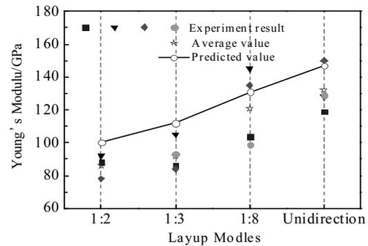
Fig.9 Predicted and experimental elastic modules in different layup modes
