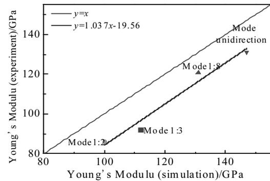
Fig.10 Comparison between experimental and simulated Young's modulus of Cf/AZ91D laminates
