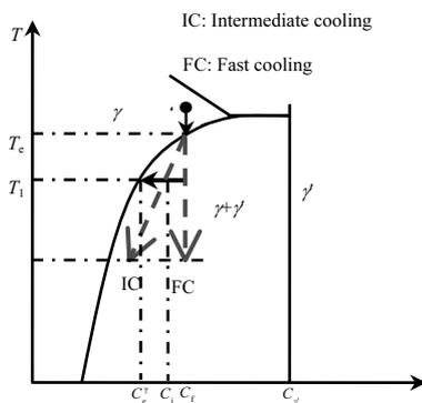
Fig.7 Illustration of Ni-Al phase diagram. Arrows describe thermodynamic paths of alloy during heat treatments consisting of continuous cooling at certain cooling rate from supersolus-solution temperature to 650 °C
