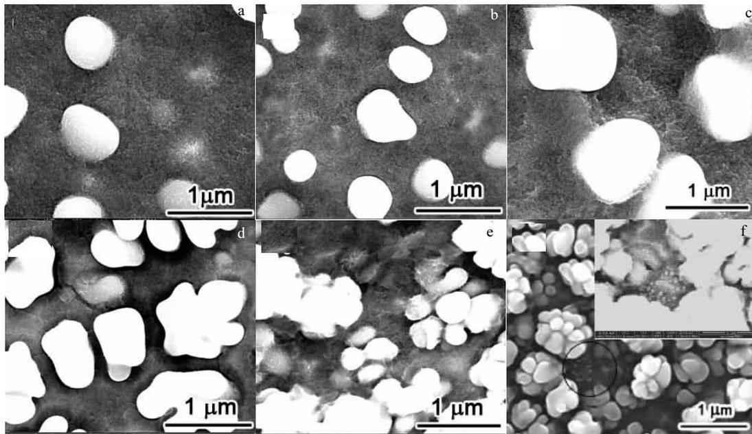
Fig.5  $\gamma'$  morphology evolution of samples subjected to isothermal heat treatments at various temperatures for 2 h: (a) 1160 °C, (b) 1125 °C, (c) 1100 °C, (d) 1050 °C, (e) 960 °C, and (f) 870 °C
