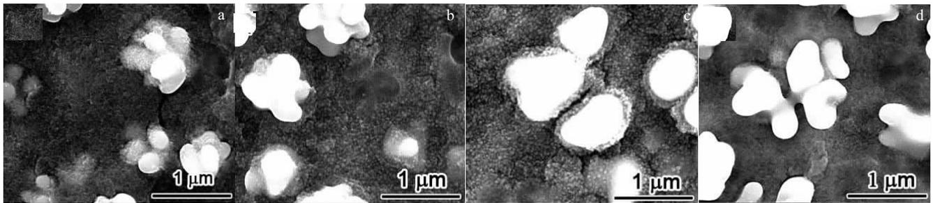
Fig.6  $\gamma'$  morphology evolution of samples subjected to isothermal heat treatments at 1125 °C for various time: (a) 5 min, (b) 15 min, (c) 30 min, and (d) 120 min
