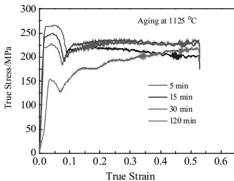
Fig.8 True stress-strain curves obtained from compression of used superalloy at 1125 °C aging for various time
