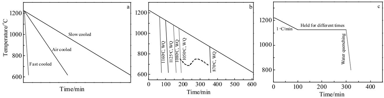
Fig.1 Illustration of continuous cooling (a), interrupted cooling tests (b), and isothermal experiments (c)
