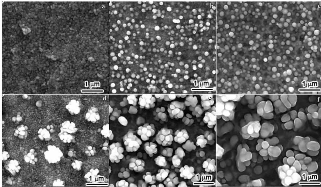
Fig.4  $\gamma'$  morphology evolution during cooling linearly at 1 °C/min and water-quenched separately at various interrupt-temperatures: (a) 1160 °C, (b) 1125 °C, (c) 1100 °C, (d) 1050 °C, (e) 960 °C, and (f) 870 °C
