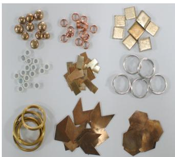
Fig.4 Morphology of the preformed filler metal
