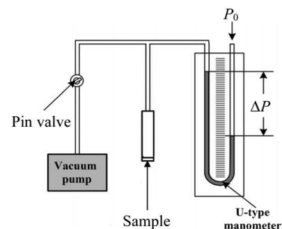
Fig.2 Schematic of the tester for gas permeability
