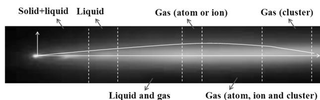
Fig.6 Photographs of PS-PVD plasma jet with 7YSZ powders injection
