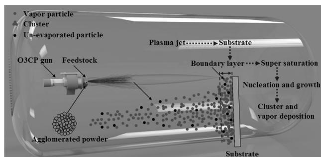
Fig.7 Schematic diagram of the nano-structured 7YSZ electrolyte layer deposited by PS-PVD
