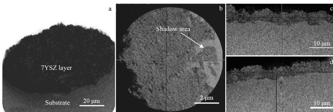
Fig.8 2D tomographies of 7YSZ electrolyte layer: (a) sample image and (b-d) different views of cross-sectional sample in Fig.8a
