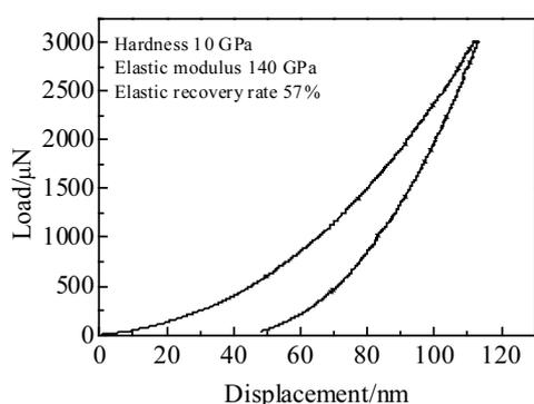
Fig.9 Loading-unloading curves of nano-structured 7YSZ
