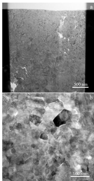
Fig.4 TEM micrographs of 7YSZ electrolyte layer
