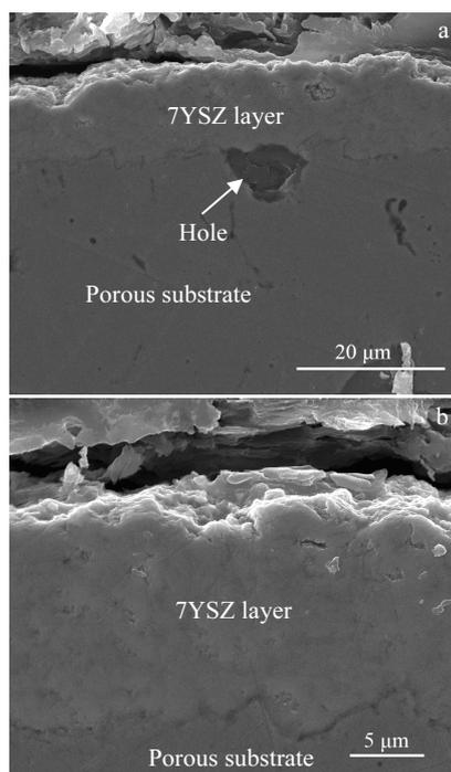
Fig.3 Cross-sectional microstructures of 7YSZ electrolyte layer on porous stainless steel 430
