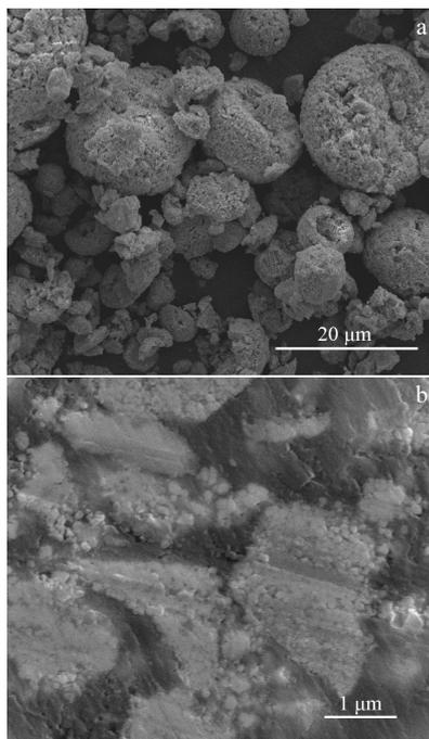
Fig.1 Morphologies of agglomerated 7YSZ powders before polishing (a) and after polishing (b)
