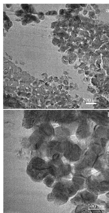
Fig.5 TEM micrographs of feedstock agglomerated 7YSZ powders before PS-PVD processing
