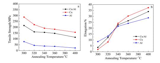
Fig.5 Variation of tensile properties of clad sheet at different annealing temperatures: (a) tensile strength and (b) elongation
