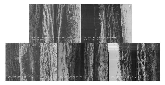
Fig.7 SEM fractographs of clad sheet at different annealing temperatures vertical to tensile axis: (a) 300 °C, (b) 320 °C, (c) 340 °C, (d) 360 °C, and (e) 400 °C
