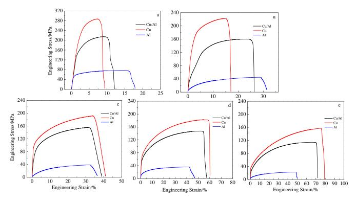
Fig.6 Engineering stress-strain curves of clad sheet and individual components at different annealing temperatures in tension tests: (a) 300 °C, (b) 320 °C, (c) 340 °C, (d) 360 °C, and (e) 400 °C
