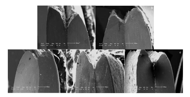
Fig.8 SEM fractographs of clad sheet at different annealing temperatures along tensile axis: (a) 300 °C, (b) 320 °C, (c) 340 °C, (d) 360 °C, and (e) 400 °C
