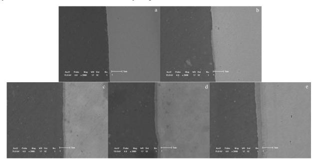
Fig.1 SEM interfacial microstructures of Cu/Al clad sheet annealed at different temperatures: (a) 300 °C, (b) 320 °C, (c) 340 °C, (d) 360 °C, and (e) 400 °C
