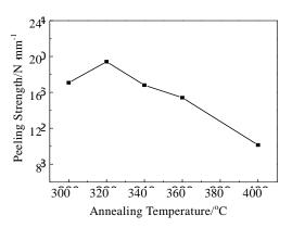
Fig.3 Variation of peeling strength of Cu/Al clad sheets with different annealing temperatures
