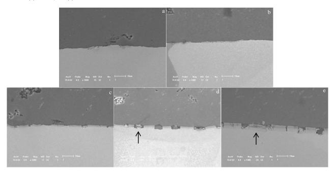
Fig.9 Interfacial microstructures of clad sheet near tensile fracture at different annealing temperatures: (a) 300 °C, (b) 320 °C, (c) 340 °C, (d) 360 °C, and (e) 400 °C
