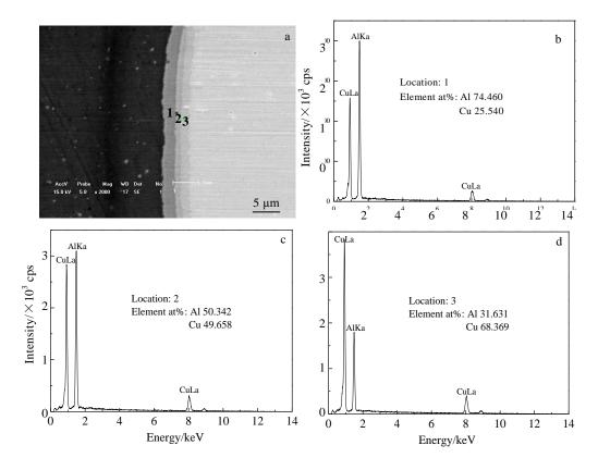
Fig.2 SEM interfacial microstructure (a) and EDS analysis results (b~d) of the interface annealed at 400 °C for 0.5 h
