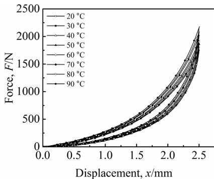
Fig.6 Hysteretic curves of common-MR at different temperatures
