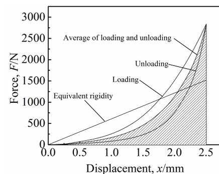
Fig.4 Solution principle of equivalent rigidity curve
