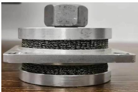
Fig.2 Picture of the SMA-MR damper
