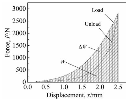
Fig.3 Hysteresis loop of the SMA-MR damping
