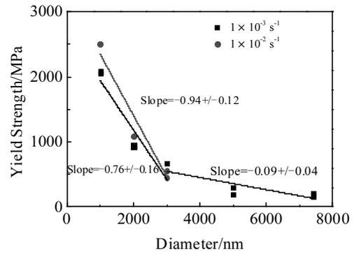
Fig.5 Relationship between yield strength of <110>-oriented single-crystalline iridium micropillars and micropillar diameters
