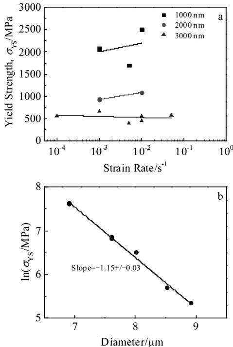
Fig.4 Yield strength of <110>-oriented single-crystalline iridium micropillars as a function of strain rate (a) and relationship between yield strength and diameters at the strain rate of  $1 \times 10^{-3} \text{ s}^{-1}$  (b)
