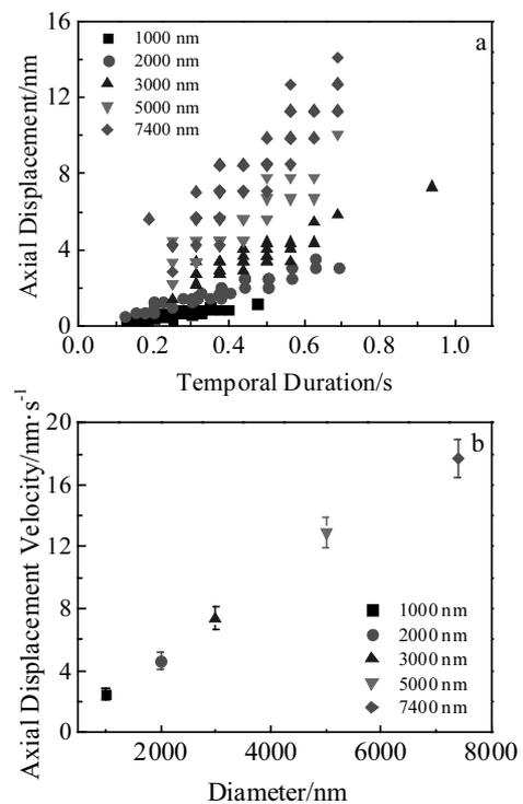
Fig.3 Relationship between axial displacement and corresponding temporal duration (a) and displacement jump velocity vs micropillar diameters (b)
