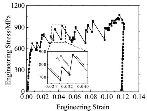
Fig.2 Engineering stress-strain curve of iridium micropillars with 3000 nm in diameter (inset displaying three zoomed-in displacement jumps)
