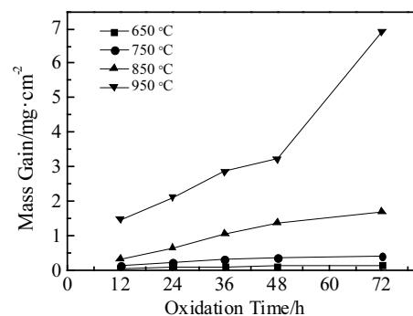
Fig.9 Oxidation kinetics curves of sintered Ti-22Al-25Nb alloy at different temperature
