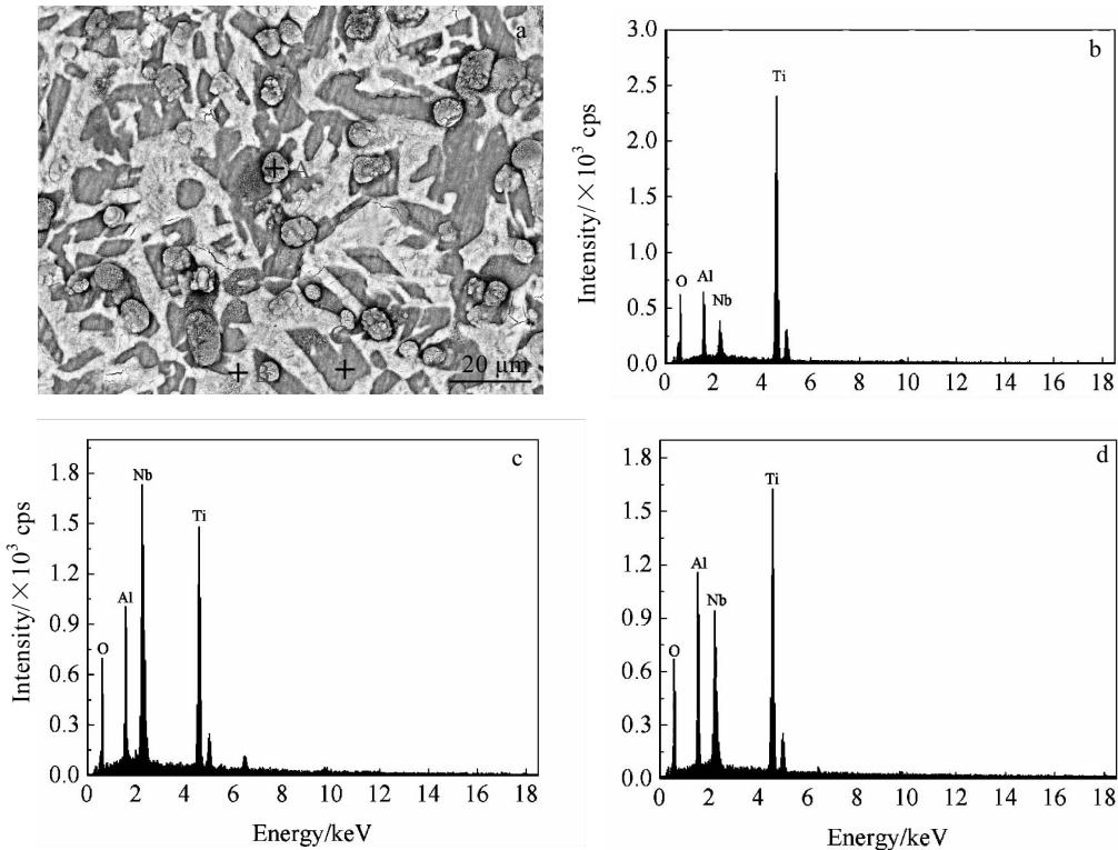
Fig.7 Typical phase composition on the surface of oxidation film: (a) BSE image, (b) EDS analysis of point A, (c) EDS analysis of point B, and (d) EDS analysis of point C
