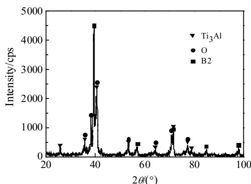
Fig.1 XRD pattern of alloy sintered at 630 °C, 20 MPa, 1 h; 1250 °C, 30 MPa, 2 h
