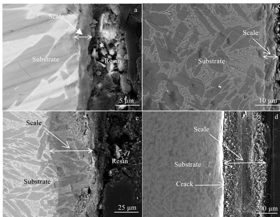
Fig.8 Cross-sectional morphologies of the samples after oxidation for 72 h at 650 °C (a), 750 °C (b), 850 °C (c), and 950 °C (d)
