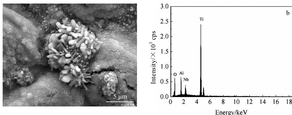
Fig.5 SEM morphology (a) and EDS analysis (b) of the typical massive particle on the oxidation film
