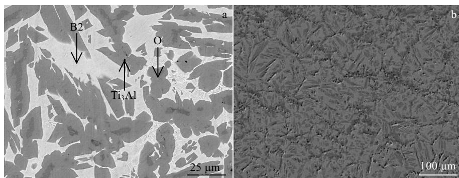
Fig.3 Microstructure of the Ti-22Al-25Nb sintered alloy: (a) BSE image, (b) SE image (the light color marks B2 phases; the grey indicates O phases; the dark grey denotes Ti<sub>3</sub>Al phases)
