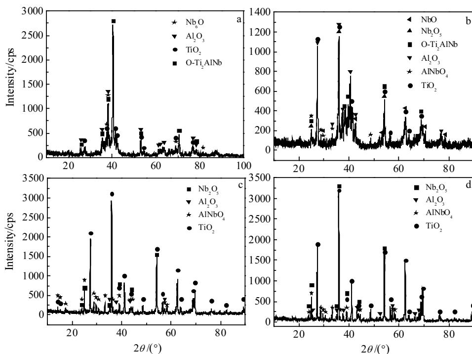
Fig.2 XRD patterns of the surface of the samples oxidized for 72 h at different temperatures: (a) 650 °C, (b) 750 °C, (c) 850 °C, and (d) 950 °C
