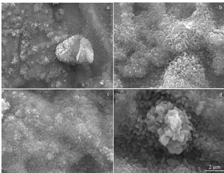
Fig.6 Surface morphologies of samples oxidized for 72 h at 650 °C (a), 750 °C (b), 850 °C (c), and 950 °C (d)
