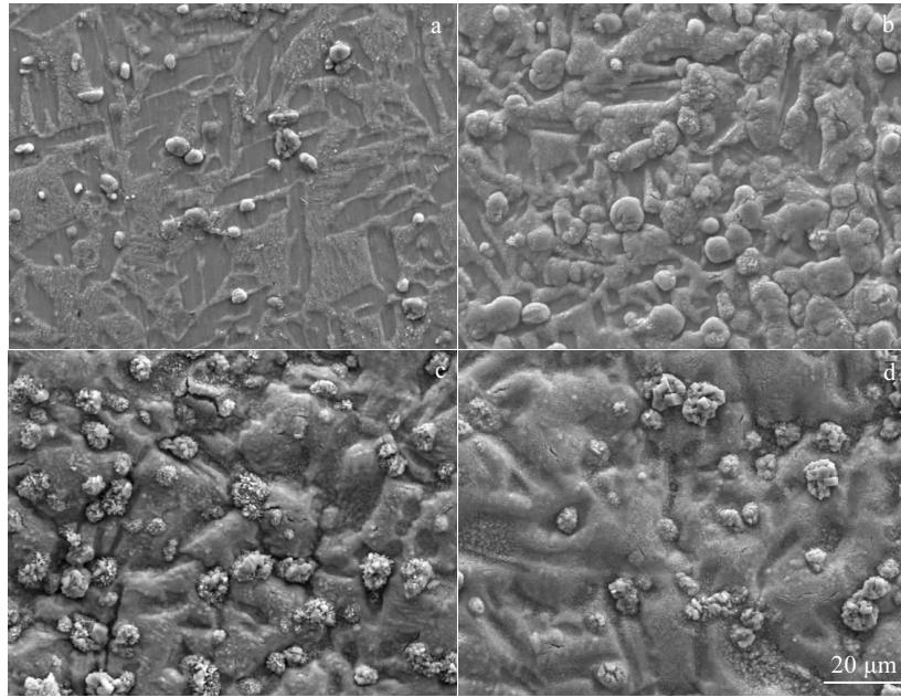
Fig.4 Surface morphologies of samples oxidized for 72 h at 650 °C (a), 750 °C (b), 850 °C (c), 950 °C (d)
