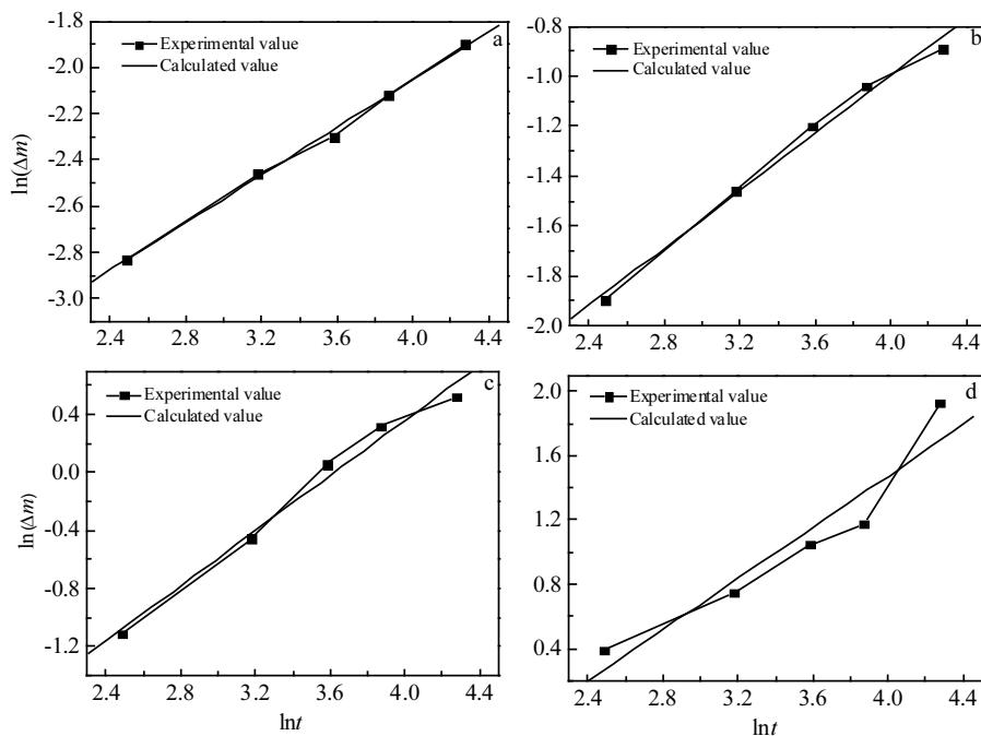
Fig.10 Oxidation kinetics curves of Ti-22Al-25Nb sintered alloy at 650 °C (a), 750 °C (b), 850 °C (c), and 950 °C (d)
