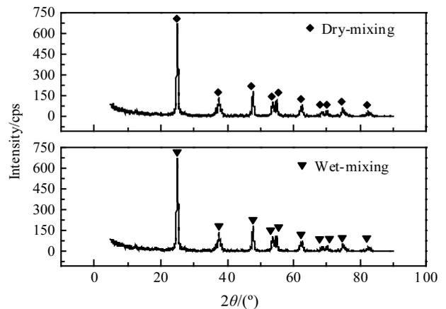
Fig.2 XRD patterns of the MWCNTs /TiO<sub>2</sub> samples
