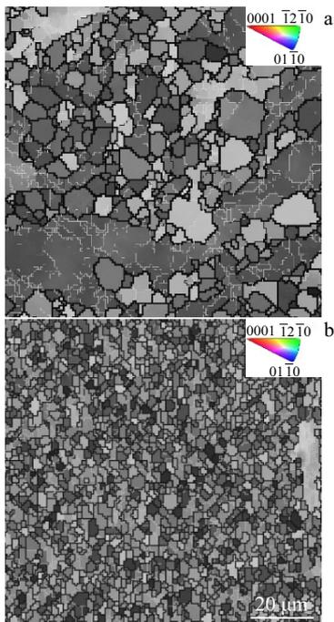
Fig.6 EBSD maps of Mg-1Zn-1Gd alloy after 4 passes (a) and 8 passes (b)
