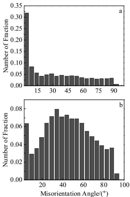
Fig.8 Misorientation angle distributions after 4 passes (a) and 8 passes (b)
