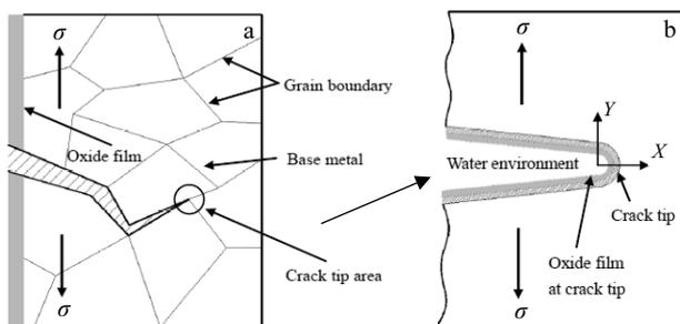
Fig.1 Diagrams of SCC intergranular propagation (a) and SCC tip (b)
