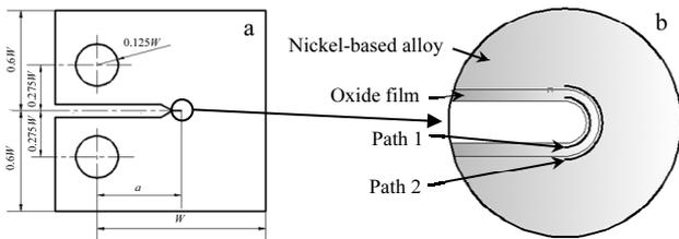
Fig.3 Specimen model: (a) geometrical shape and size of 1T-CT specimen ( $W=50$  mm,  $a=0.5W$ ,  $c=1.6$  mm) and (b) SCC tip and measured paths
