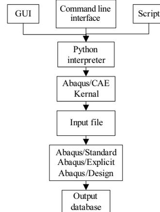
Fig.5 Procedure of ABAQUS
