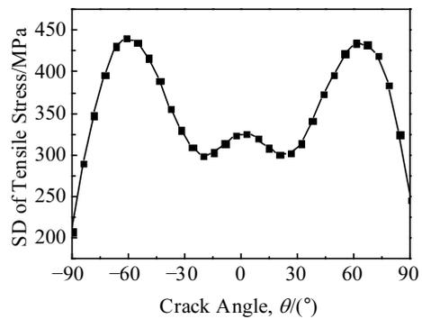
Fig.8 SD of tensile stress along path 1
