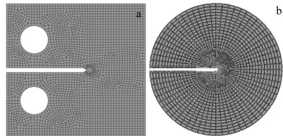
Fig.4 Finite element mesh of 1T-CT specimen: (a) whole model and (b) detail around cracking tip
