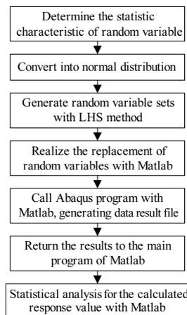
Fig.6 Block diagram of joint program of MATLAB and ABAQUS
