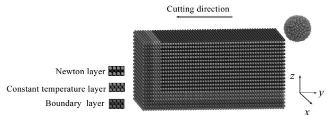
Fig.2 Molecular dynamics model of nano-cutting single crystal  $\gamma$ -TiAl alloy
