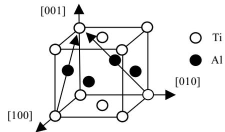
Fig.1 Lattice structure of  $\gamma$ -TiAl alloy
