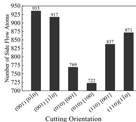
Fig.8 Comparison of the number of side flow atoms along different cutting crystal directions
