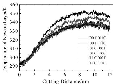
Fig.5 Curves of temperature change of Newton layer in workpiece along different cutting crystal orientations
