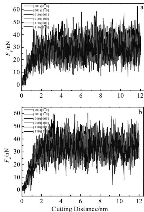
Fig.4 Curves of main cutting force  $F_y$  (a) and normal cutting force  $F_z$  (b) along different cutting directions
