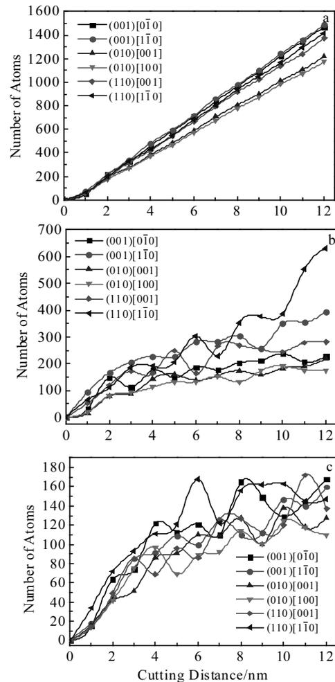
Fig.10 Number of atoms for transformation of dfcc (a), hcp (b), and bcc (c) lattice structures along different cutting directions
