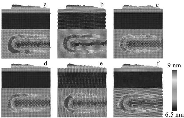
Fig.6 Surface morphologies of workpiece cut along (001)[010] (a), (001)[110] (b), (010)[001] (c), (010)[100] (d), (110)[001] (e), and (110)[110] (f) crystal orientations
