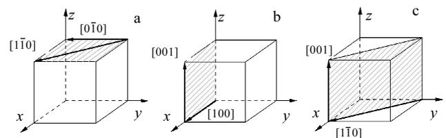
Fig.3 Schematic diagram of cutting direction on (001) (a), (010) (b), and (110) (c) crystal planes of single crystal  $\gamma$ -TiAl alloy
