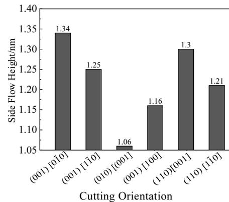
Fig.7 Comparison of lateral flow heights along different cutting crystal directions
