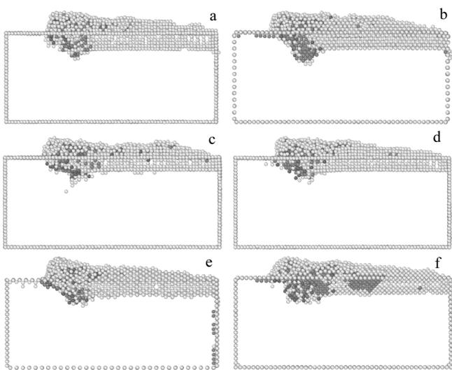
Fig.9 Structures of cutting layer of workpiece cut along  $(001)[0\bar{1}0]$ (a),  $(001)[1\bar{1}0]$ (b),  $(010)[001]$ (c),  $(010)[100]$ (d),  $(110)[001]$ (e), and  $(110)[1\bar{1}0]$ (f) crystal orientations
