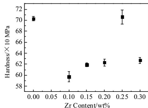
Fig.5 Vickers micro-hardness of Al-Mn-Fe 3104 alloys with different Zr contents
