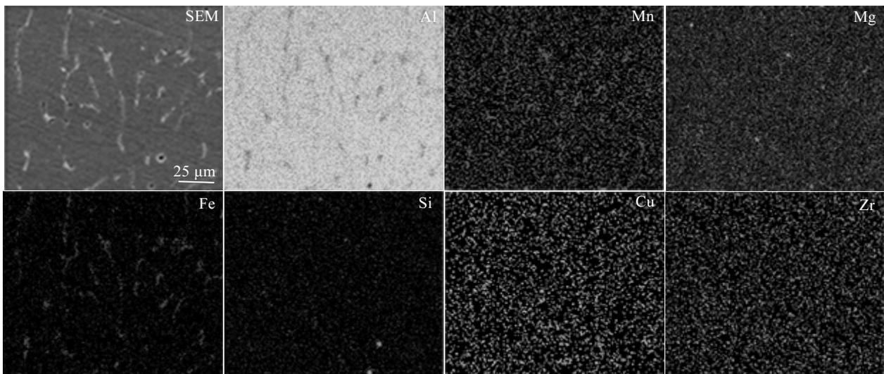
Fig.3 SEM microstructure and EDS analysis of 3104 aluminium alloy with 0.2wt% Zr
