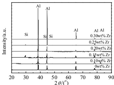
Fig.4 XRD patterns of the Al-Mn-Fe 3104 alloys with different Zr contents
