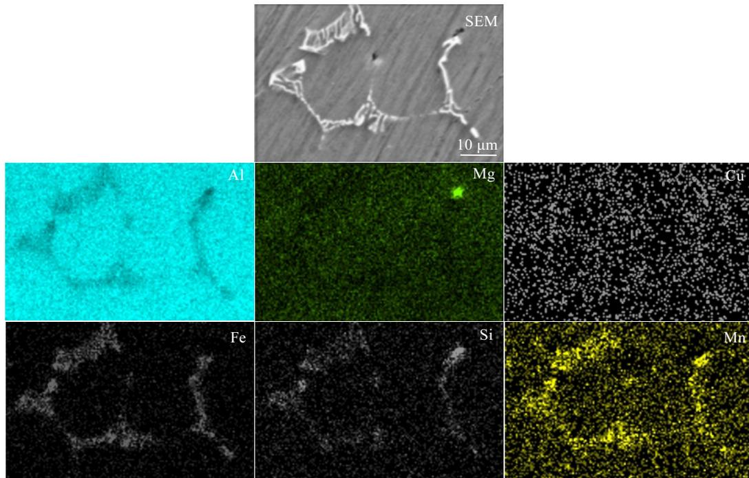
Fig.2 SEM microstructure and EDS analysis of industrial Al-Mn-Fe 3104 alloy without Zr
