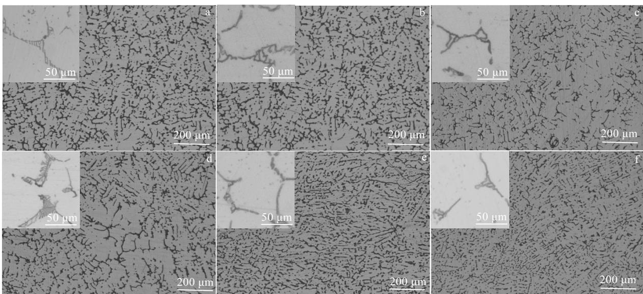
Fig.1 OM micrographs of Al-Mn-Fe 3104 alloys with different Zr additions: (a) 0wt%, (b) 0.10wt%, (c) 0.15wt%, (d) 0.20wt%, (e) 0.25wt%, and (f) 0.30wt%
