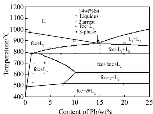
Fig.1 Calculated isopleth at 14 wt% Sn in the copper-rich part of the Cu-Sn-Pb system<sup>[21]</sup>
