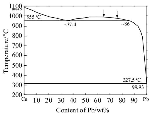
Fig.3 Phase diagram of Cu-Pb monotectic alloy<sup>[23]</sup>
