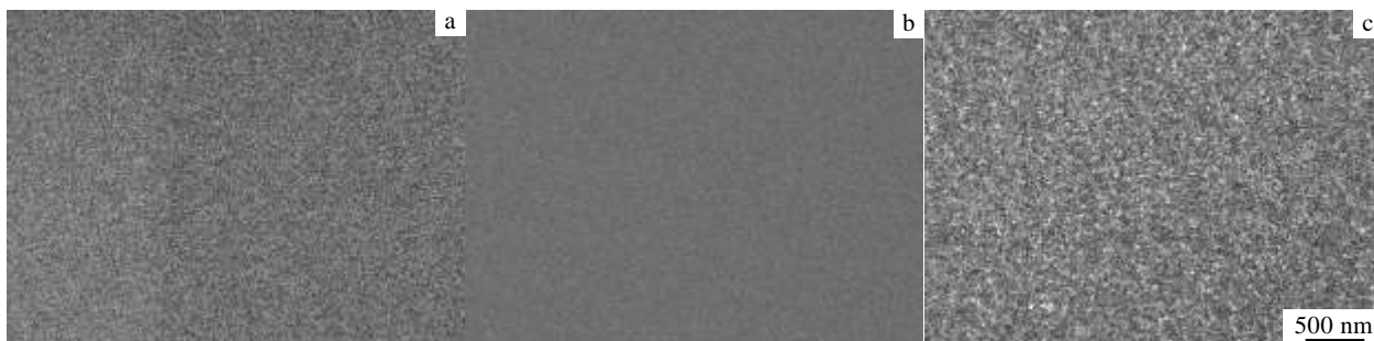
Fig.3 SEM images of Ti(C,N,O) films deposited under different gas mixture flow rates: (a) 10 mL/min, (b) 50 mL/min, and (c) 80 mL/min
