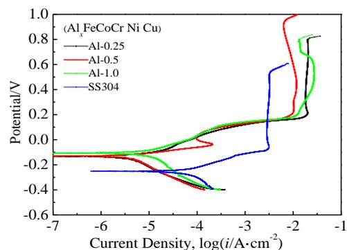
Fig.4 Polarization curves for HEA coatings and SS 304 stainless steel in 0.5 mol/L H<sub>2</sub>SO<sub>4</sub> solution
