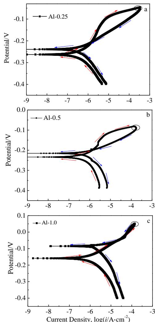
**Fig.5** Cyclic polarization curves for Al<sub>0.25</sub>FeCoCrNiCu (a) Al<sub>0.5</sub>FeCoCrNiCu (b), and Al<sub>1.0</sub>FeCoCrNiCu (c) in 1 mol/L NaCl solution**Table 3 Polarization parameters of HEA coatings in 1 mol/L NaCl solution**
