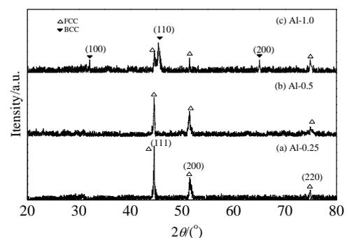
**Fig.1** XRD patterns of HEA coatings ( $\text{Al}_x\text{FeCoCrNiCu}$ )
