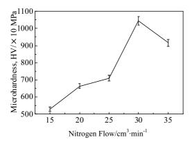
Fig.5 Impact of nitrogen flow on microhardness of CrN films
