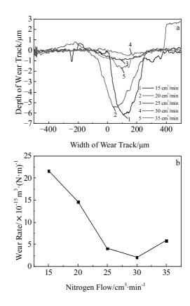
Fig.7 Sectional profile of the wear track (a) and wear rate (b) of CrN films
