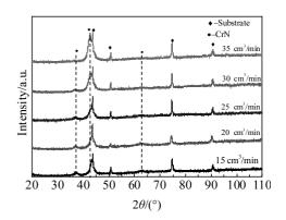
Fig.4 XRD patterns of CrAlN films at different nitrogen flow
