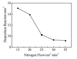
Fig.3 Deposition rate of CrN films as a function of nitrogen flow
