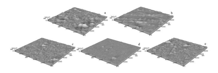
Fig.2 AFM images and roughness of CrN films at different nitrogen flow: (a) 15 cm<sup>3</sup>/min,  $R_a$ =11.7 nm; (b) 20 cm<sup>3</sup>/min,  $R_a$ =10.7 nm; (c) 25 cm<sup>3</sup>/min,  $R_a$ =6.53 nm; (d) 30 cm<sup>3</sup>/min,  $R_a$ =4.77 nm; (e) 35 cm<sup>3</sup>/min,  $R_a$ =10.4 nm
